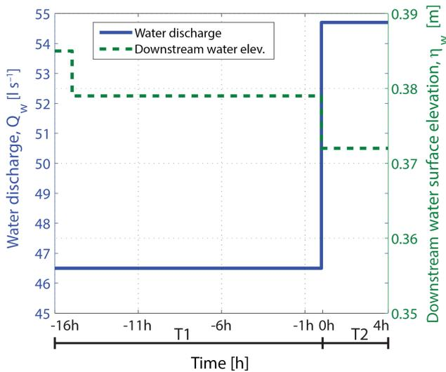
**Figure 2.** Water discharge,  $Q_w$ , and base level (i.e., water surface elevation at the downstream end),  $\eta_w$ , imposed in Experiments T<sub>1</sub> and T<sub>2</sub>. The water surface elevation was measured at  $x = 10.62$  m.
