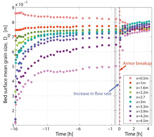
**Figure 10.** Measured change in the geometric mean grain size of the bed surface sediment at various locations in Experiments T<sub>1</sub> and T<sub>2</sub>. The blue dotted line indicates the moment of the increase in flow rate ( $t = 0$  h) and the red dashed line indicates the moment of armor breakup ( $t = 4$  min).
