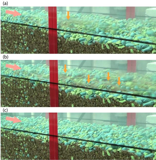
**Figure 8.** Armor breakup and reformation between Compartments 6 and 7: (a) initial local breakup, (b) widening of the breakup and exposure of the finer substrate, (c) reformation of the mobile armor. Flow is from left to right. Blurriness in images (a) and (b) indicates the entrainment of sand (orange arrows).
