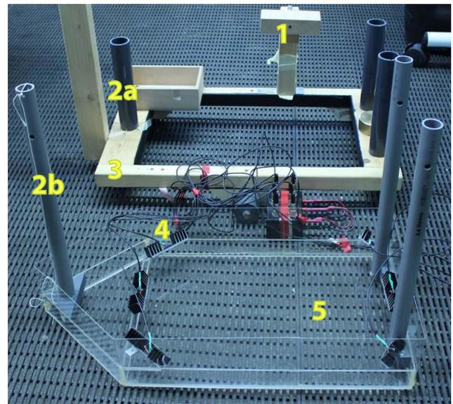
**Figure 4.** Floating part of the equipment for measuring the grain size distribution of the bed surface during the laboratory experiments. Here the bottom and the walls of the floating part are made of thin Plexiglas® plates and higher Plexiglas® sheets are attached along the walls to avoid water overflow. The numbers indicate (1) position of the camera, (2a) upper pipe, (2b) lower pipe, (3) carriage, (4) LED light attached to the cooling plate, and (5) floating part.
