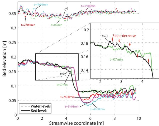
**Figure 6.** Measured water surface and bed elevation profiles of Experiment T<sub>2</sub> at  $t = 0$  h 07 min, 2 h 08 min, 3 h 08 min, and 4 h 08 min. The enlarged window shows the degradation occurring during the armor breakup. Flow is from left to right. The profiles were smoothed using a Gaussian filter.
