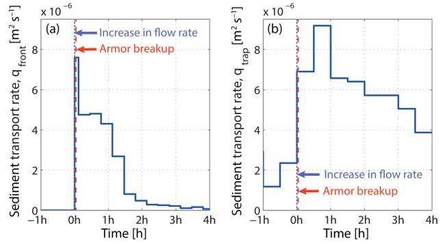
**Figure 12.** Measured sediment transport rate (a) computed from the migration of the front between the trimodal reach and the sand reach using Eq. (1), (b) at the downstream end of the flume. Horizontal line intervals indicate time-averaged values.
