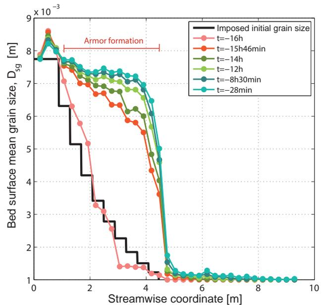
**Figure 5.** Imposed and measured geometric mean grain size of the bed surface sediment at various times for Experiment T<sub>1</sub>.
