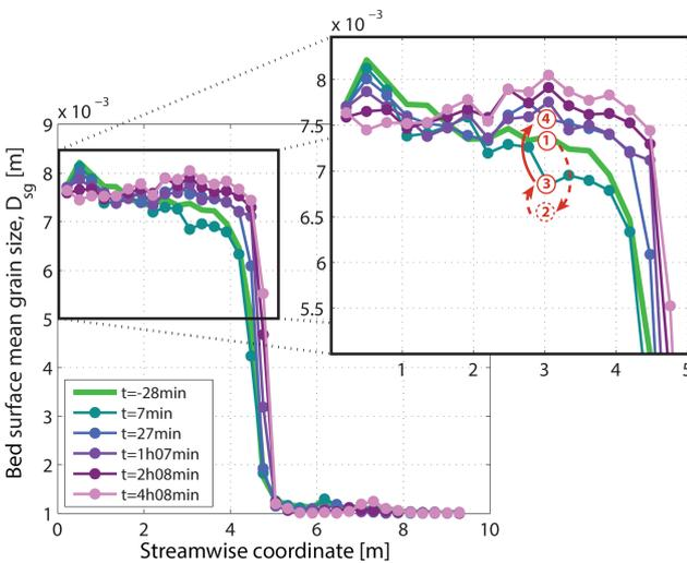
**Figure 9.** Measured geometric mean grain size of the bed surface sediment at various times for Experiment T<sub>2</sub>. Points 1 to 4 in the enlarged window show the temporal change in the bed surface. Point 2 indicates a hypothetical (i.e., not measured; see Fig. 8b) finer surface at the moment of the breakup. Point 3 corresponds to the coarser bed surface shown in Fig. 8c right after the reformation of the armor.
