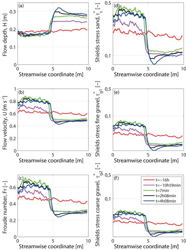
**Figure 11.** Hydraulic conditions of experiment  $T_1$  and  $T_2$ : (a) flow depth, (b) flow velocity, (c) Froude number, (d) Shields stress for the sand fraction (logarithmic scale), (e) Shields stress for the fine gravel fraction (logarithmic scale), and (f) Shields stress for the coarse gravel fraction (logarithmic scale). The Shields stress values were determined accounting for a sidewall correction due to Vanoni and Brooks (1957).
