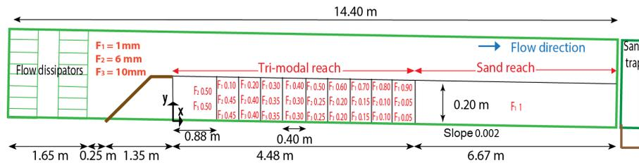
**Figure 1.** Flume setup and initial bed for Experiment T<sub>1</sub>. The red numbers indicate the volumetric gravel fraction content in each compartment.
