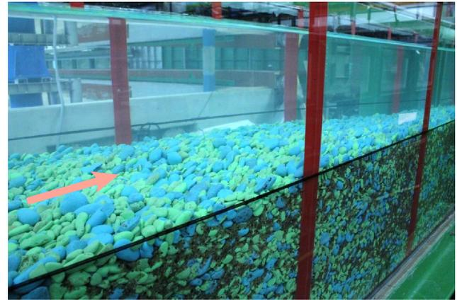
**Figure 7.** Imbrication of the bed surface sediment at the end of Experiment T<sub>1</sub>. Flow is from left to right.
