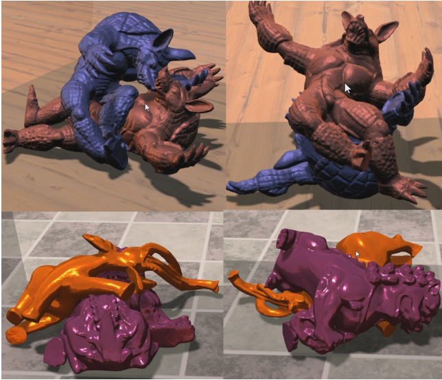
Fig. 2. Interactive simulations of complex elastic deformables with contact in real-time. Collisions and self-intersections are naturally handled.
