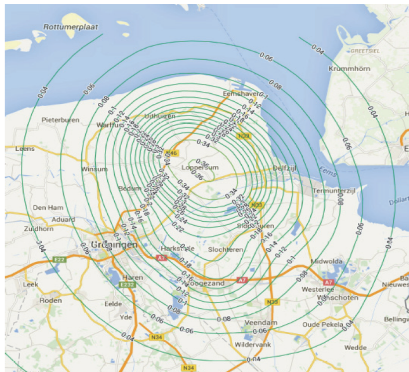
Figure 3.5: Probabilistic seismic hazard map for Groningen using V0 GMPEs, for a return period of 475 years and a period of T=0.01 s. The contour lines indicate the PGA zones (max PGA is 0.36 g near Loppersum) (source: Spetzler and Dost, 2016 in NPR 9998, 2015 ).
