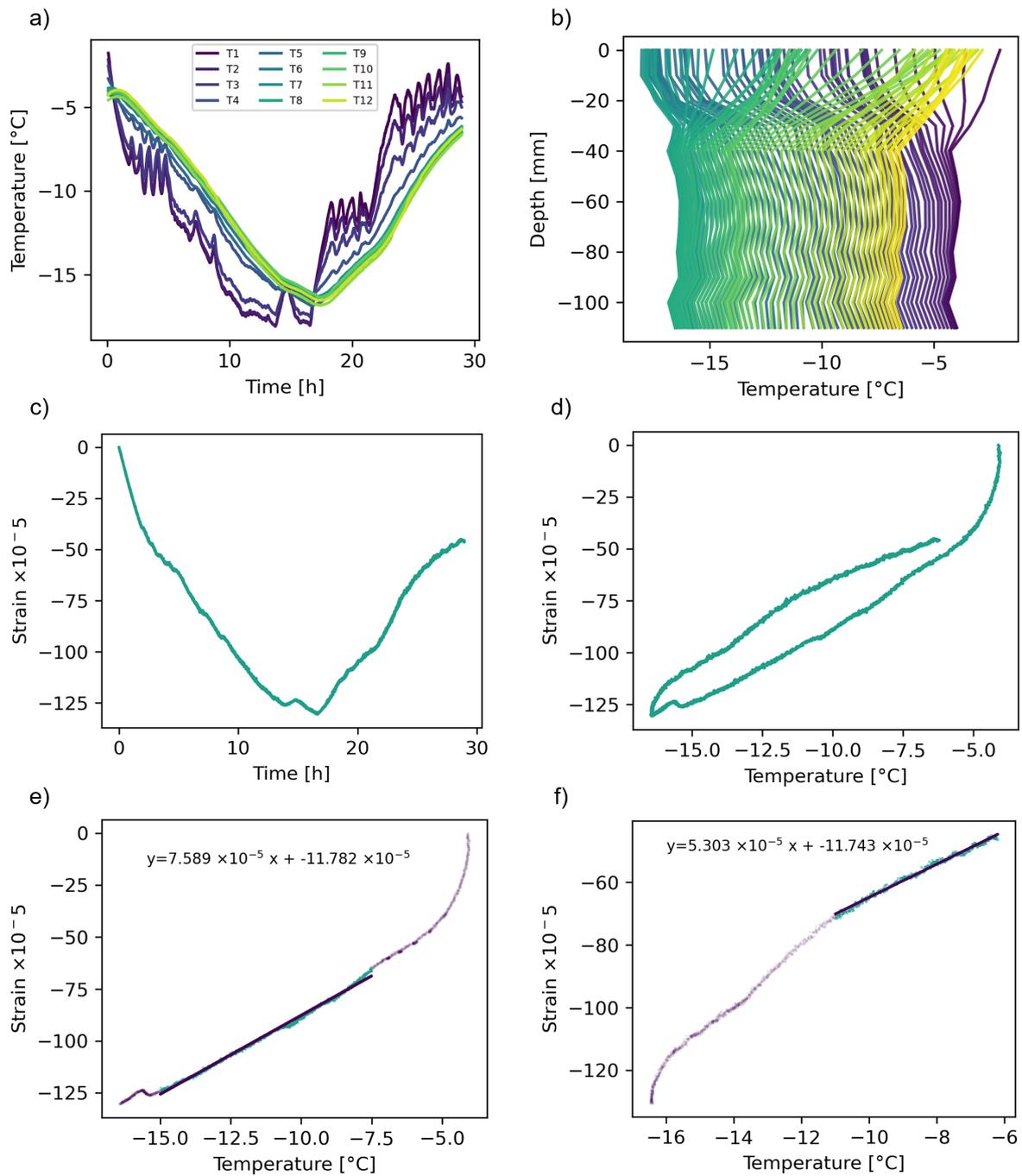
Figure A.5: **Experiment E04**, fresh ice on the table, sample 01B1. (a) Temperature profile, cooling then heating (b) Temperature gradient (c) Strain over time (d) Strain over mean ice temperature (e-f) Strain over mean ice temperature ECTE calculation. The slope of the line equates to the ECTE value for the experiment.
