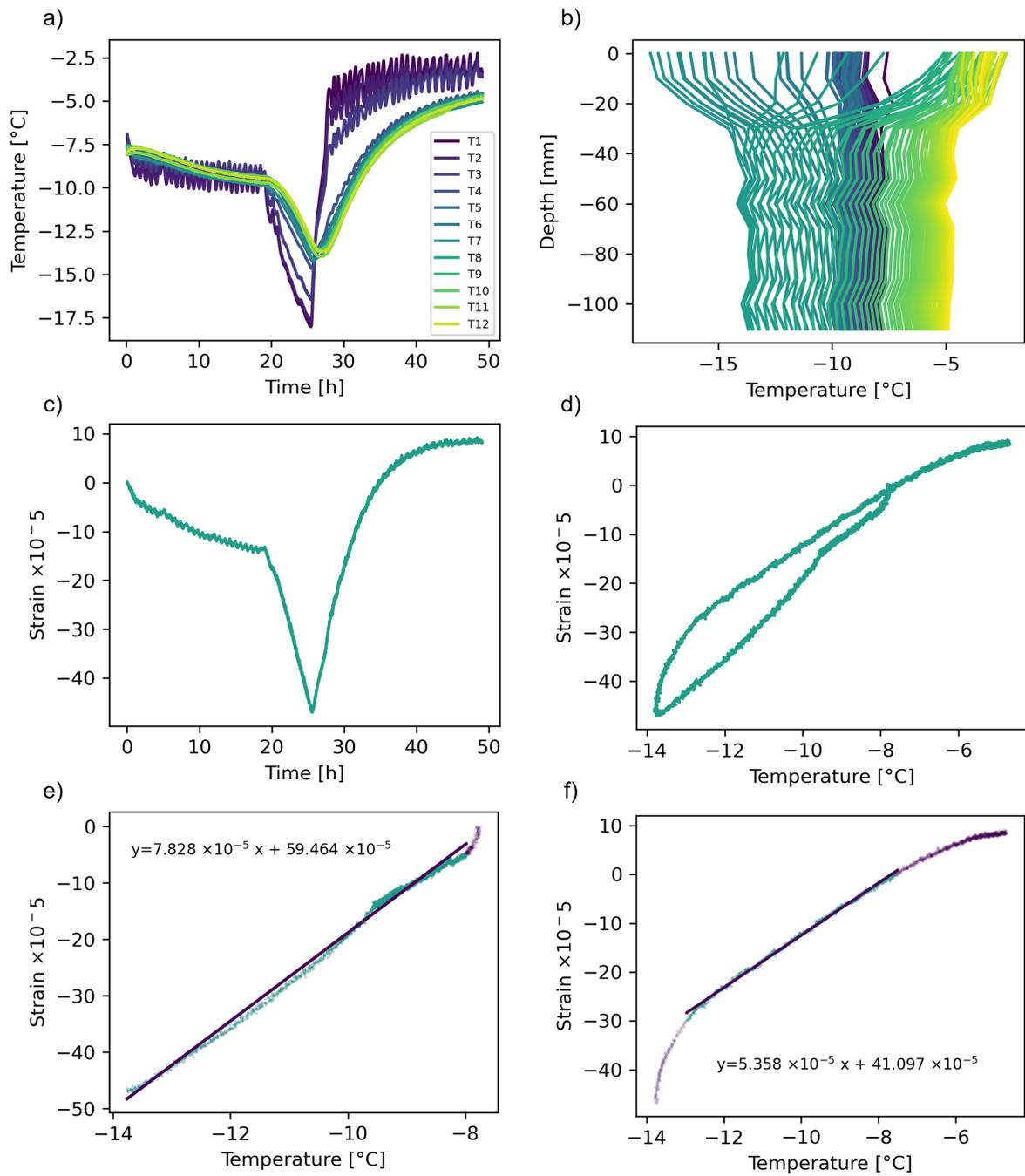
Figure A.13: **Experiment E12**, granular saline ice on the table, sample 02A1. (a) Temperature profile, cooling then heating (b) Temperature gradient (c) Strain over time (d) Strain over mean ice temperature (e-f) Strain over mean ice temperature ECTE calculation. The slope of the line equates to the ECTE value for the experiment.
