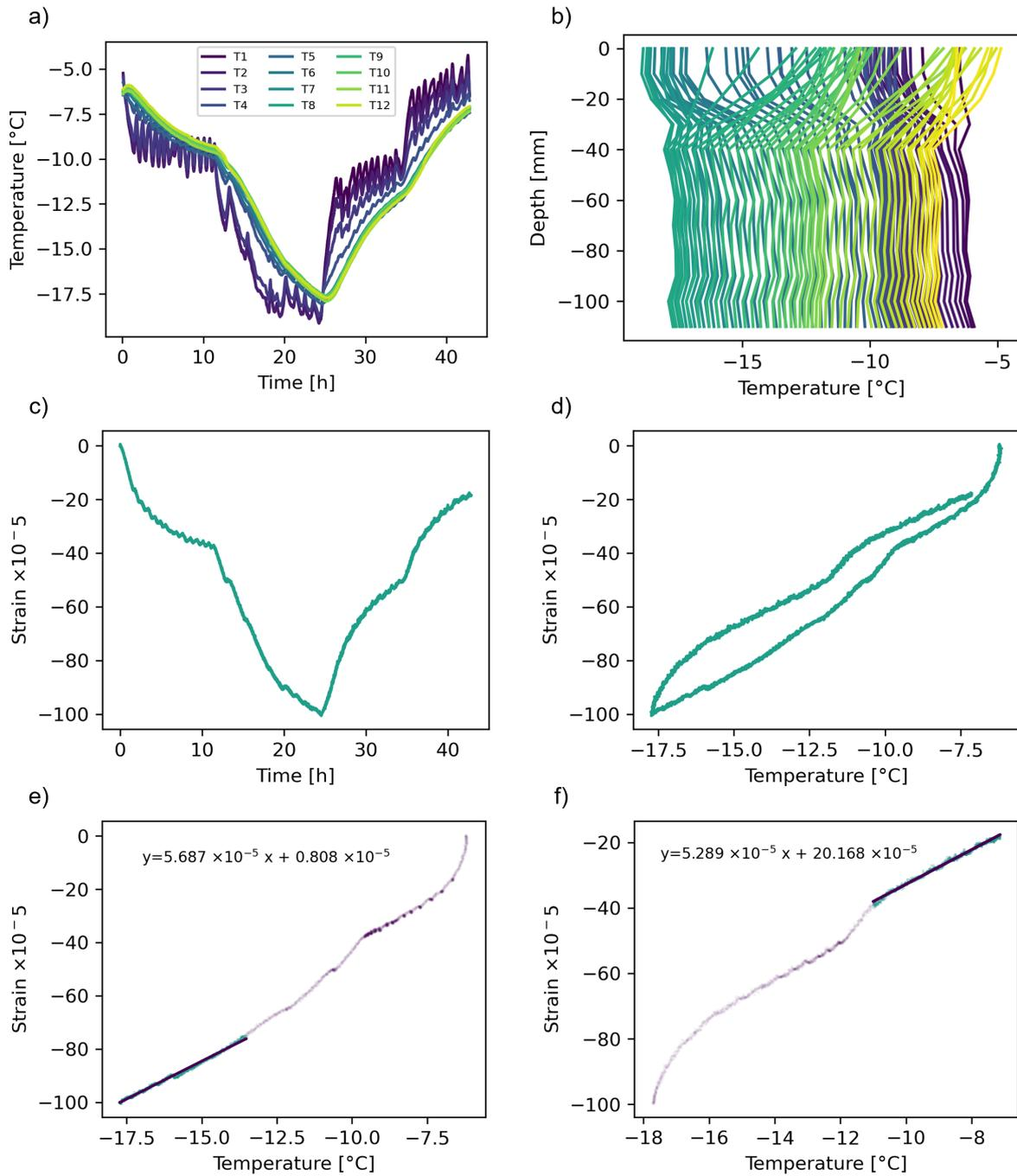
Figure A.6: **Experiment E05**, fresh ice on the table, sample 01B1. (a) Temperature profile, cooling then heating (b) Temperature gradient (c) Strain over time (d) Strain over mean ice temperature (e-f) Strain over mean ice temperature ECTE calculation. The slope of the line equates to the ECTE value for the experiment.
