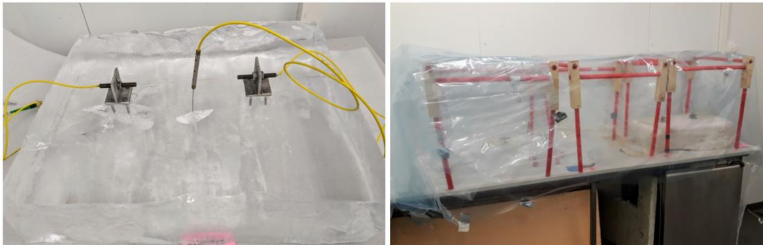
(a) Sample 01A1 and FBG strain and temperature sensor set-up.
