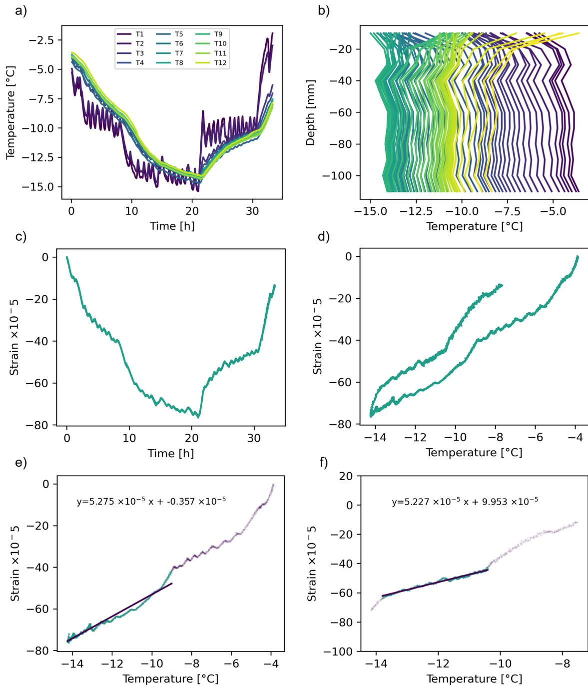
Figure A.9: **Experiment E08**, fresh ice on the table, sample 01B1. (a) Temperature profile, cooling then heating (b) Temperature gradient (c) Strain over time (d) Strain over mean ice temperature (e-f) Strain over mean ice temperature ECTE calculation. The slope of the line equates to the ECTE value for the experiment.
