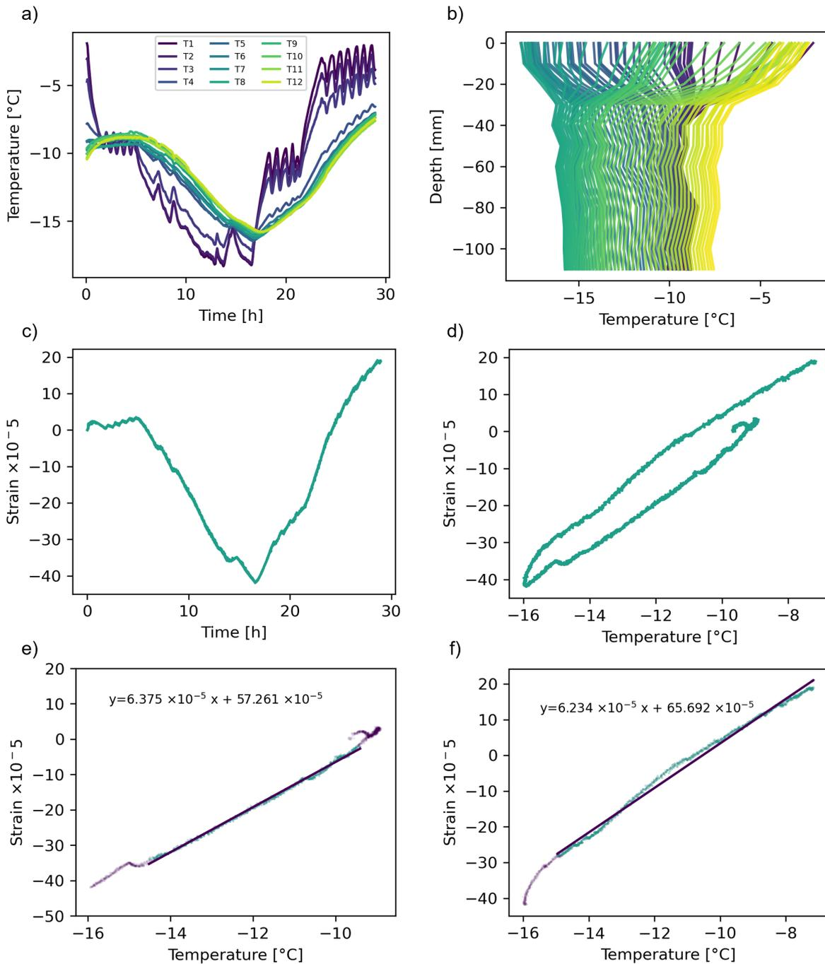
Figure A.11: **Experiment E10**, granular saline ice on the table, sample 02A1. (a) Temperature profile, cooling then heating (b) Temperature gradient (c) Strain over time (d) Strain over mean ice temperature (e-f) Strain over mean ice temperature ECTE calculation. The slope of the line equates to the ECTE value for the experiment.
