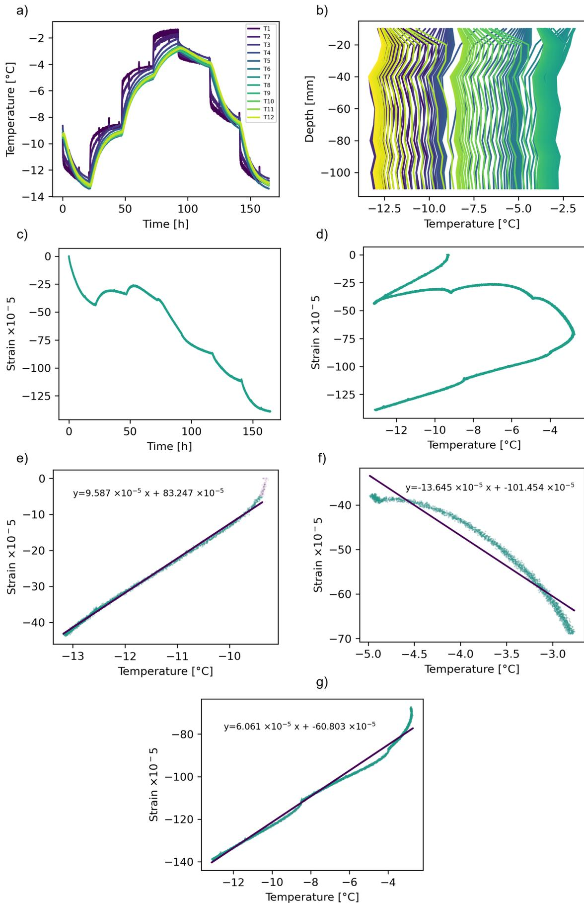
Figure A.15: **Experiment E13**, Svea ice on the table, sample 03A1, depth of 20 cm below the ice surface. (a) Temperature profile, cooling then heating then cooling (b) Temperature gradient (c) Strain over time (d) Strain over mean ice temperature (e-g) Strain over mean ice temperature ECTE calculation. The slope of the line equates to the ECTE value for the experiment.
