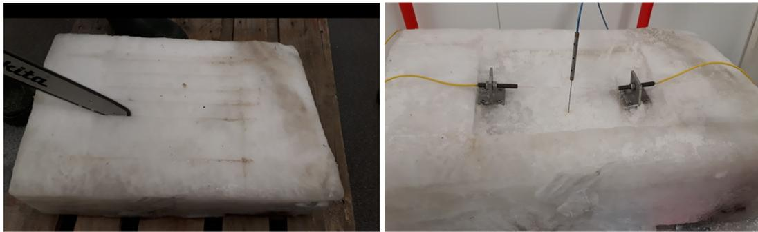
(a) Method for constructing pool in granular saline ice sample with chainsaw. (b) Empty pool in saline ice sample before seawater was added.
