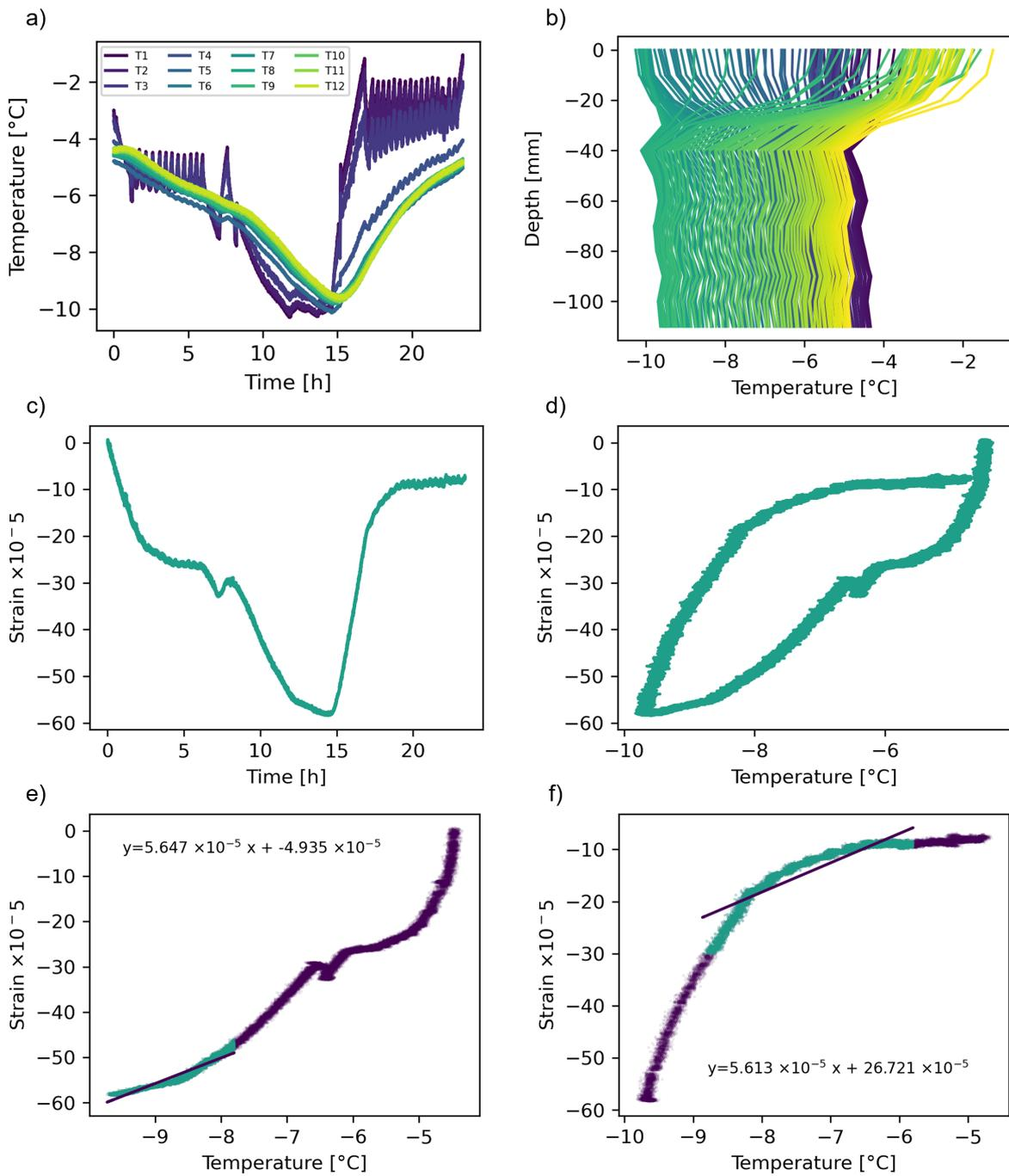
Figure A.4: **Experiment E03**, fresh ice on the table, sample 01A1. (a) Temperature profile, cooling then heating (b) Temperature gradient (c) Strain over time (d) Strain over mean ice temperature (e-f) Strain over mean ice temperature ECTE calculation. The slope of the line equates to the ECTE value for the experiment.
