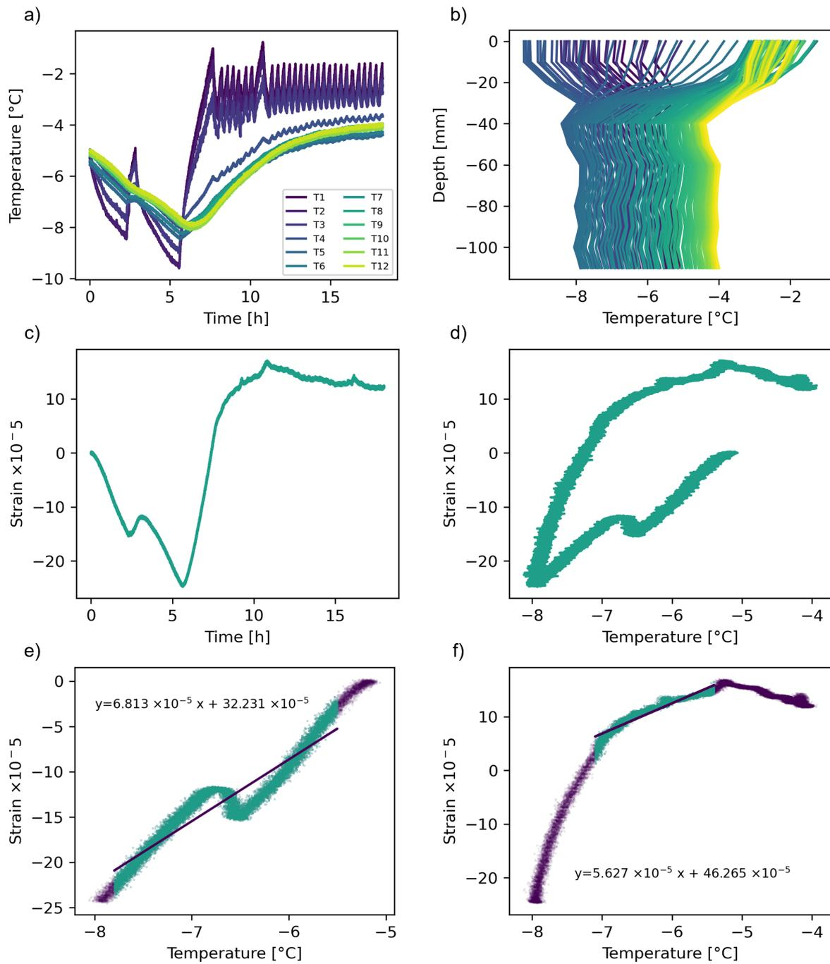
Figure A.2: Part two of **Experiment E01**, fresh ice on the table, sample 01A1. (a) The temperature profile of cooling then heating (b) Temperature gradient (c) Strain over time (d) Strain over mean ice temperature (e-f) Strain over mean ice temperature ECTE calculation. The slope of the line equates to the ECTE value for the experiment.
