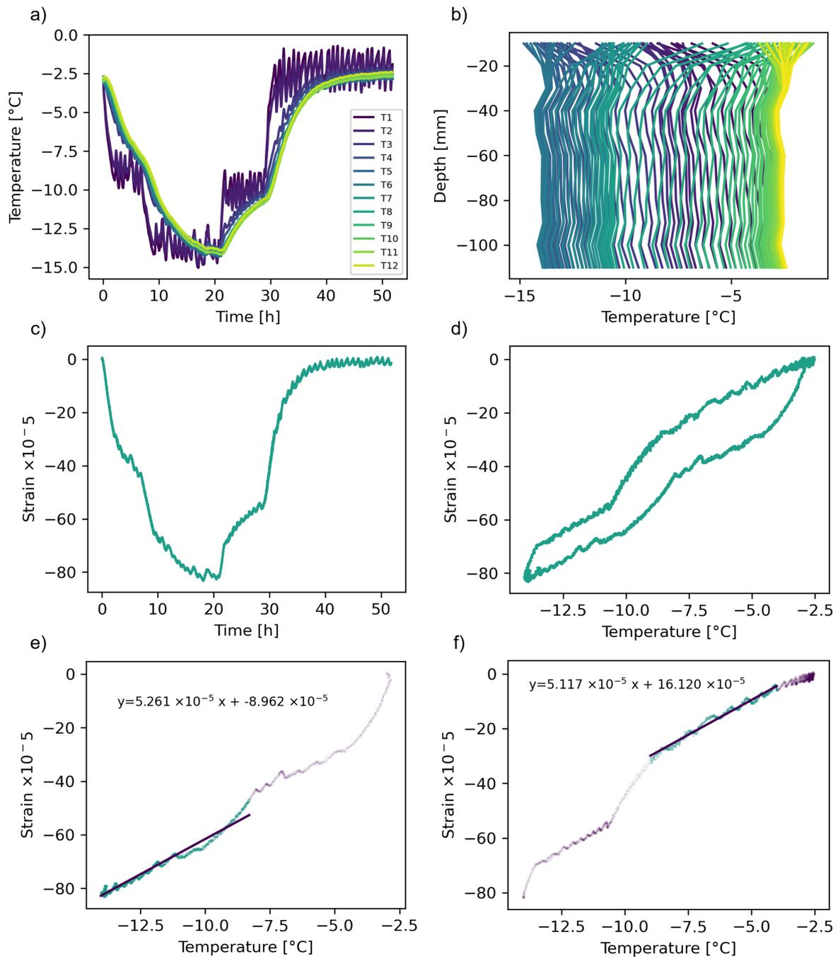
Figure A.10: **Experiment E09**, fresh ice on the table, sample 01B1. (a) Temperature profile, cooling then heating (b) Temperature gradient (c) Strain over time (d) Strain over mean ice temperature (e-f) Strain over mean ice temperature ECTE calculation. The slope of the line equates to the ECTE value for the experiment.
