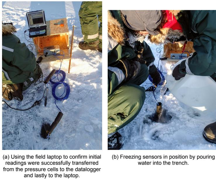
Figure 3.20: Svea fieldwork equipment installation.
