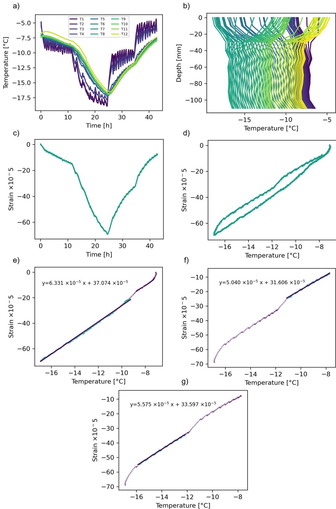
Figure A.12: **Experiment E11**, granular saline ice on the table, sample 02A1. (a) Temperature profile, cooling then heating (b) Temperature gradient (c) Strain over time (d) Strain over mean ice temperature (e-g) Strain over mean ice temperature ECTE calculation. The slope of the line equates to the ECTE value for the experiment.
