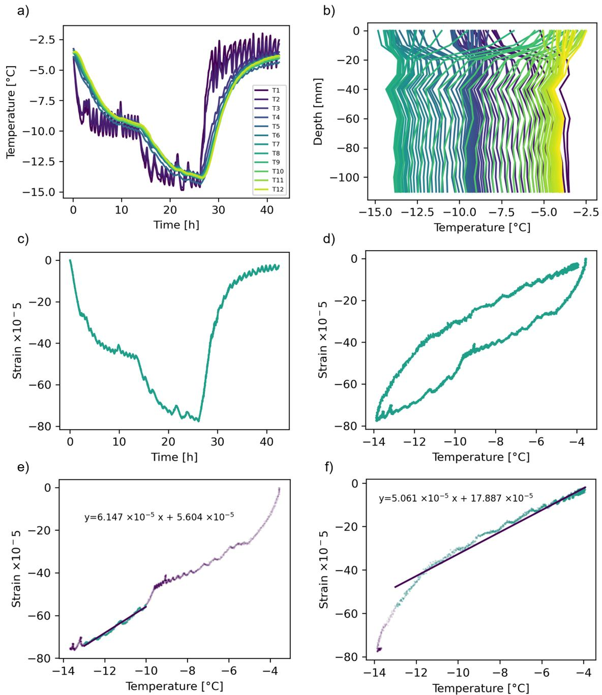
Figure A.8: **Experiment E07**, fresh ice on the table, sample 01B1. (a) Temperature profile, cooling then heating (b) Temperature gradient (c) Strain over time (d) Strain over mean ice temperature (e-f) Strain over mean ice temperature ECTE calculation. The slope of the line equates to the ECTE value for the experiment.
