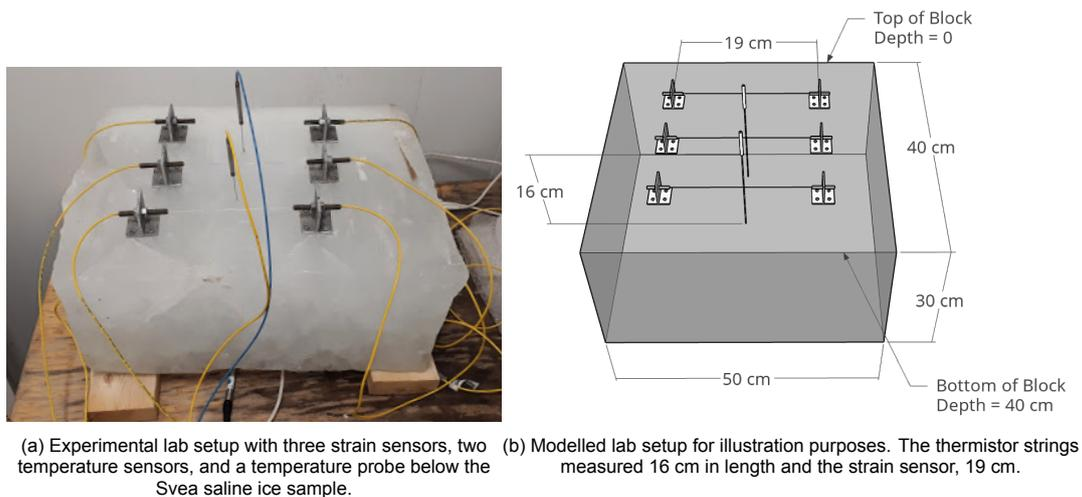
(a) Experimental lab setup with three strain sensors, two temperature sensors, and a temperature probe below the Svea saline ice sample. (b) Modelled lab setup for illustration purposes. The thermistor strings measured 16 cm in length and the strain sensor, 19 cm.
