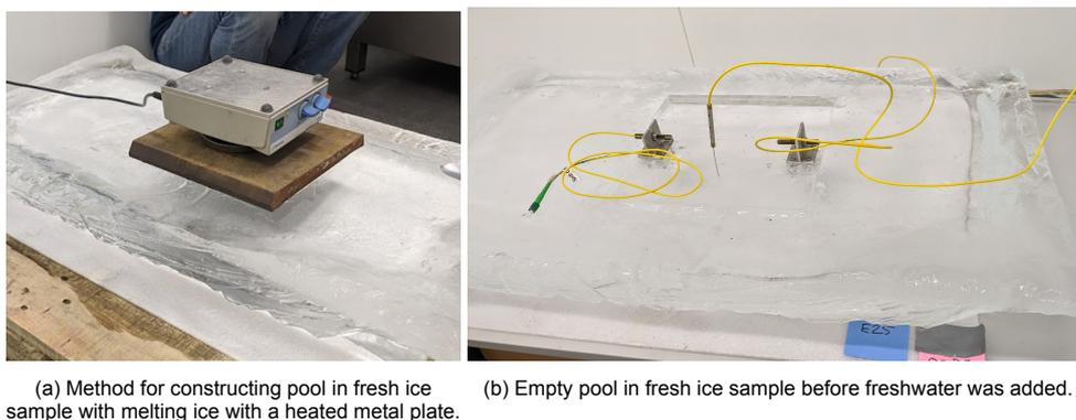
(a) Method for constructing pool in fresh ice sample with melting ice with a heated metal plate. (b) Empty pool in fresh ice sample before freshwater was added.
