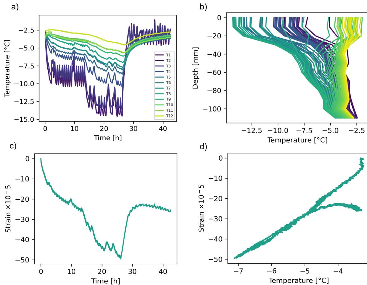
Figure A.24: **Experiment E21**, Floating granular saline ice, sample 02A1. (a) Temperature profile, cooling then heating (b) Temperature gradient (c) Strain over time (d) Strain over mean ice temperature
