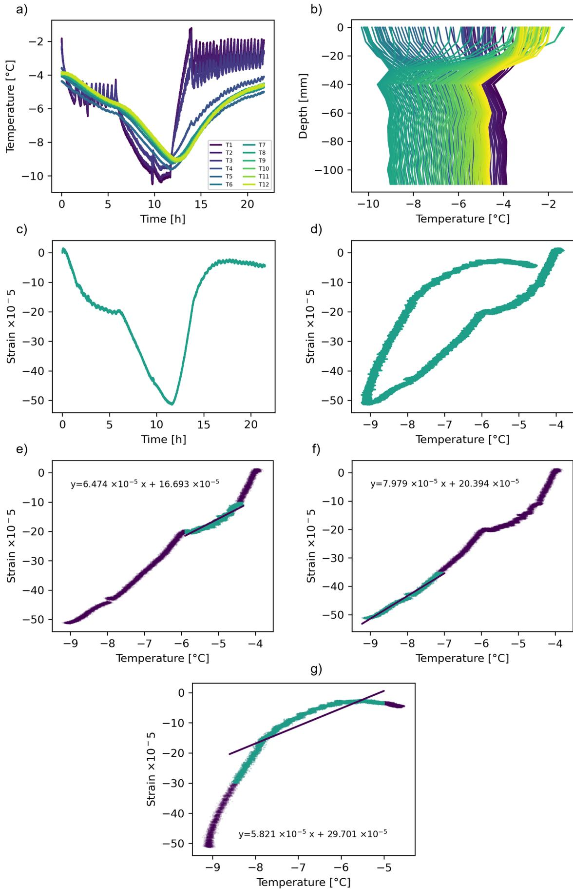
Figure A.3: **Experiment E02**, fresh ice on the table, sample 01A1. (a) Temperature profile, cooling then heating (b) Temperature gradient (c) Strain over time (d) Strain over mean ice temperature (e-g) Strain over mean ice temperature ECTE calculation. The slope of the line equates to the ECTE value for the experiment.
