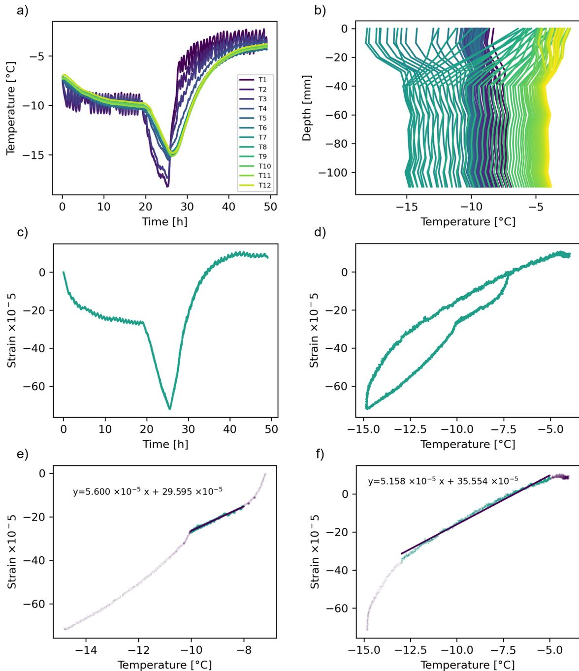
Figure A.7: **Experiment E06**, fresh ice on the table, sample 01B1. (a) Temperature profile, cooling then heating (b) Temperature gradient (c) Strain over time (d) Strain over mean ice temperature (e-f) Strain over mean ice temperature ECTE calculation. The slope of the line equates to the ECTE value for the experiment.
