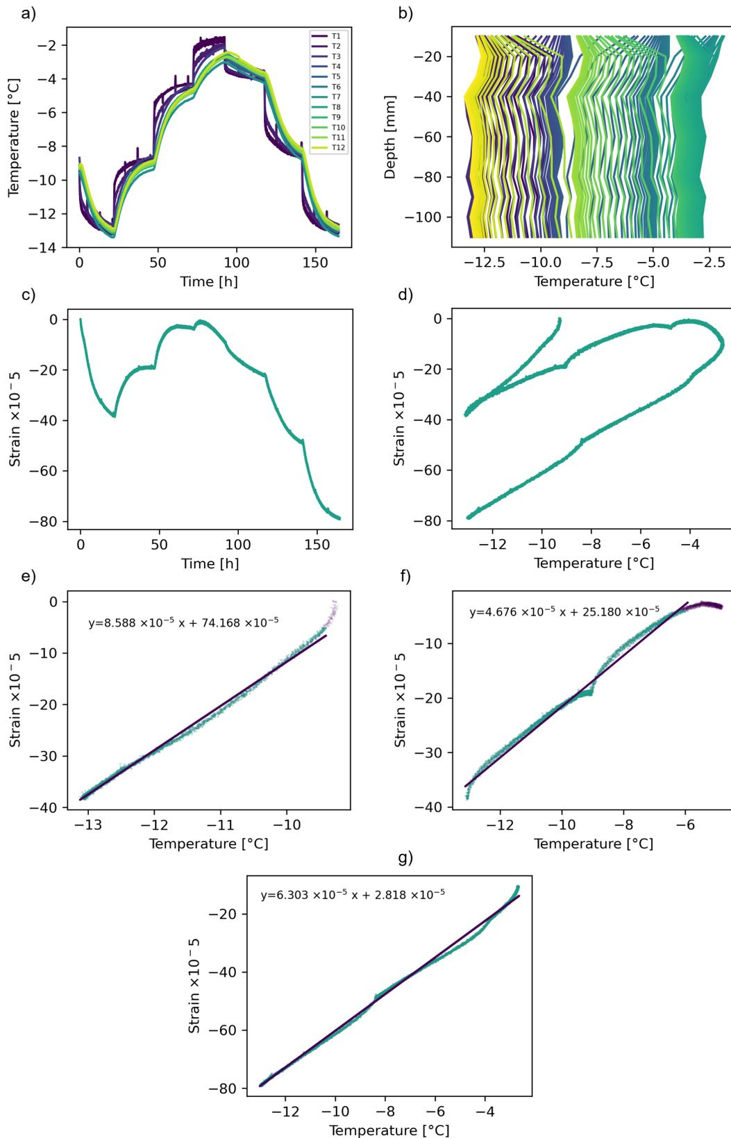
Figure A.14: **Experiment E13**, Svea ice on the table, sample 03A1, depth of 10 cm below the ice surface. (a) Temperature profile, cooling then heating then cooling (b) Temperature gradient (c) Strain over time (d) Strain over mean ice temperature (e-g) Strain over mean ice temperature ECTE calculation. The slope of the line equates to the ECTE value for the experiment.
