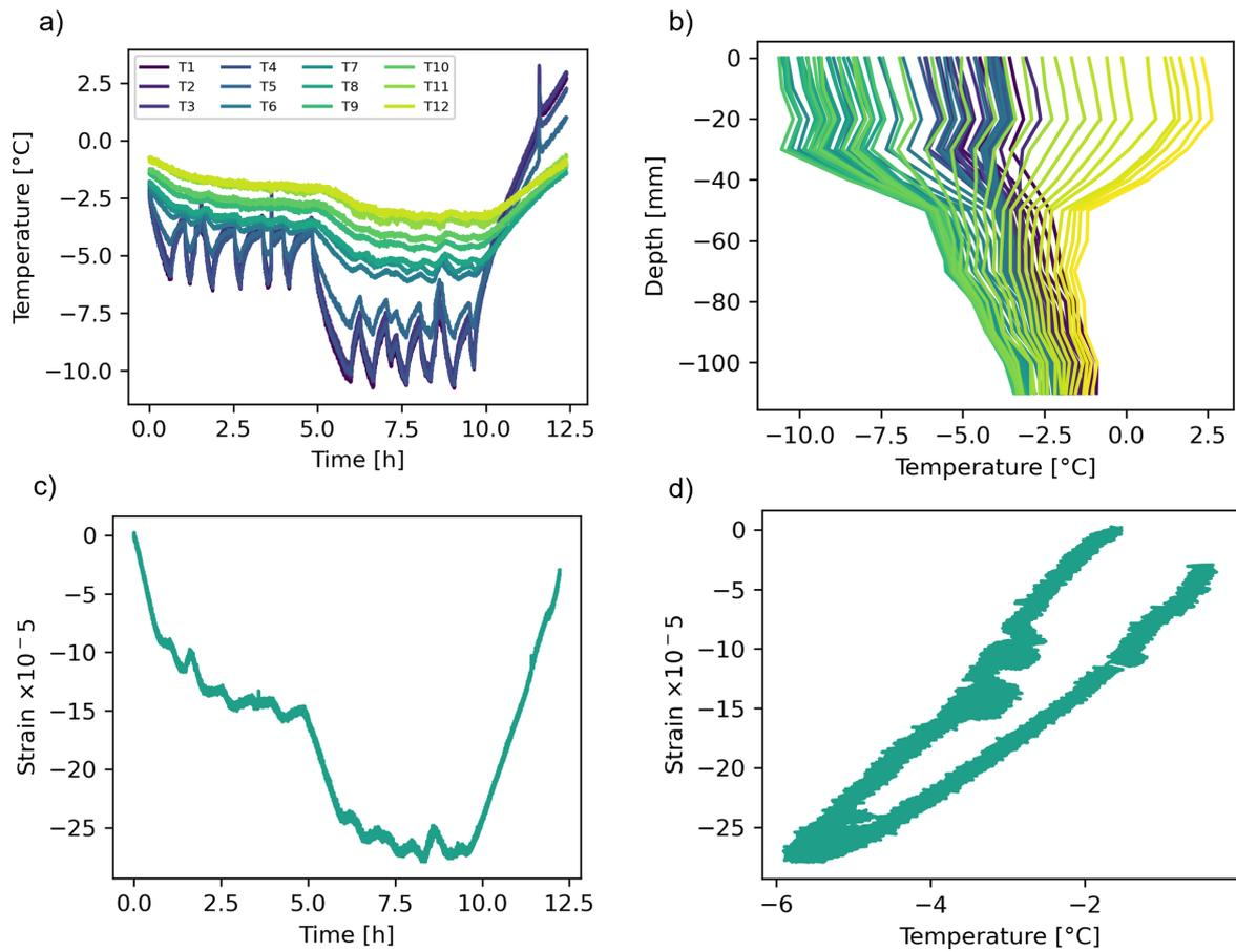
Figure A.21: **Experiment E18**, Floating fresh ice, sample 01B1. (a) Temperature profile, cooling then heating (b) Temperature gradient (c) Strain over time (d) Strain over mean ice temperature (TS5 to TS12)
