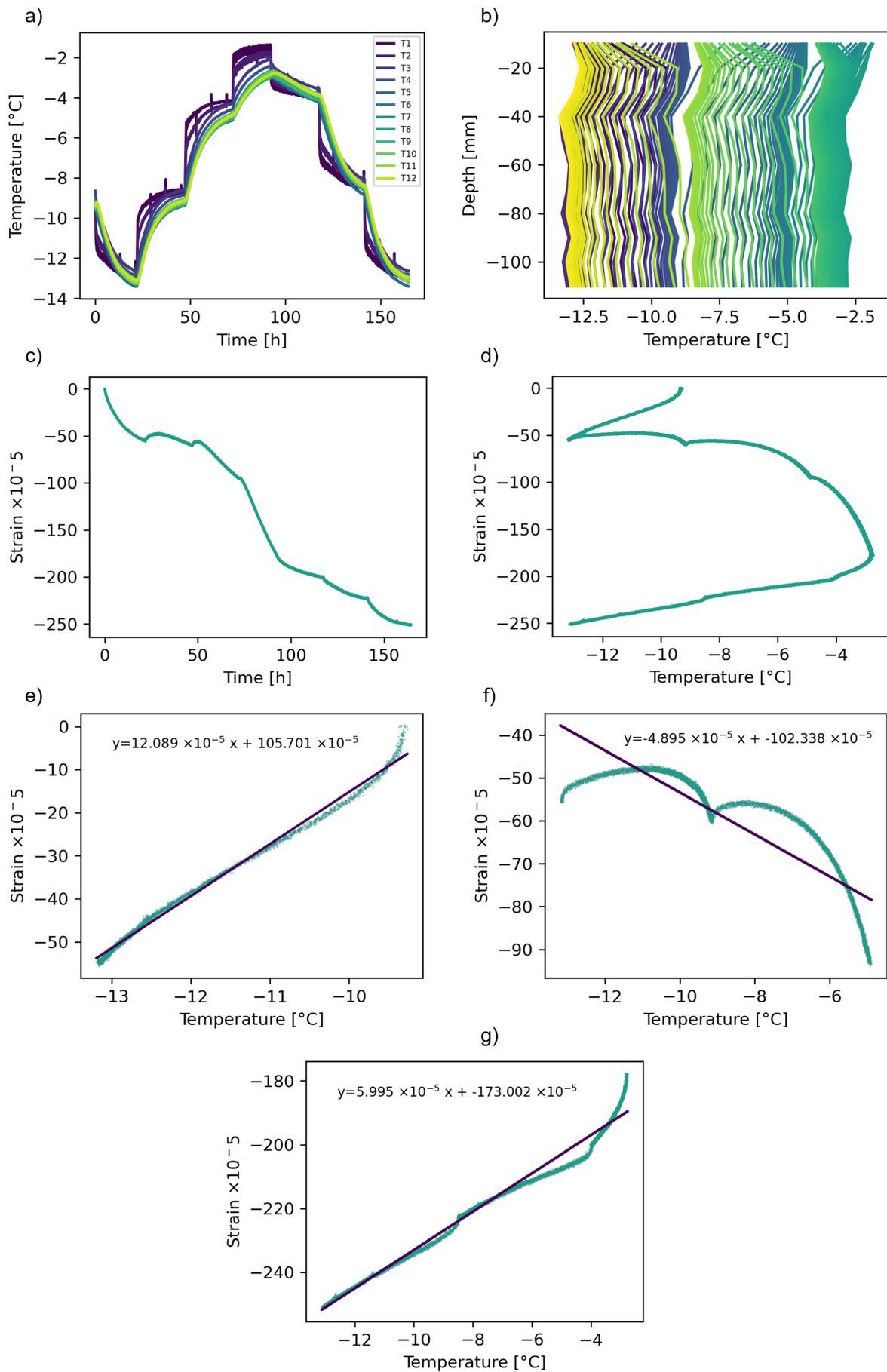
Figure A.16: **Experiment E13**, Svea ice on the table, sample 03A1, depth of 30 cm below the ice surface. (a) Temperature profile, cooling then heating then cooling (b) Temperature gradient (c) Strain over time (d) Strain over mean ice temperature ECTE calculation. The slope of the line equates to the ECTE value for the experiment. (e-g) Strain over mean ice temperature ECTE calculation. Negative ECTE values were found in this test.
