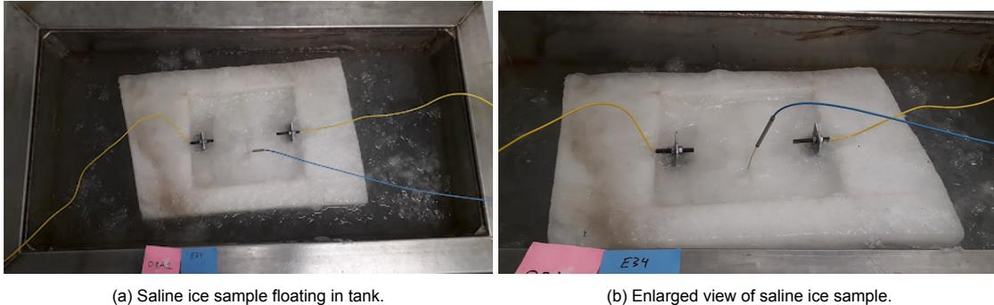
Figure 3.15: Floating unconfined saline ice thermal expansion experiment.
