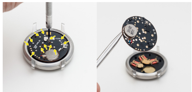
Figure 16. Removal of PCB and Stepper motors 39
