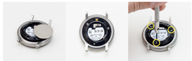
Figure 15. Battery removal and access to the PCB 39
