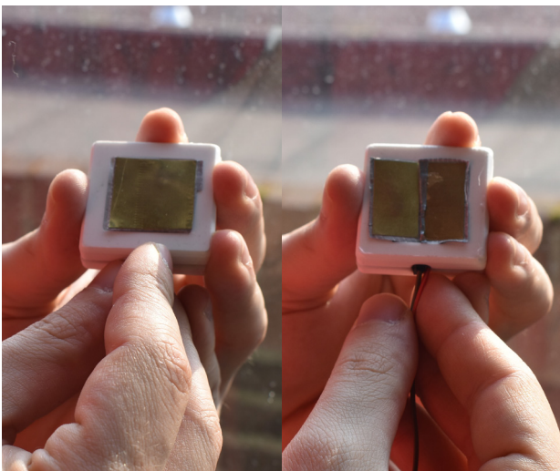
Figure 75. Necklace prototype to test against the chest. Two electrodes on one side, one on the other.
