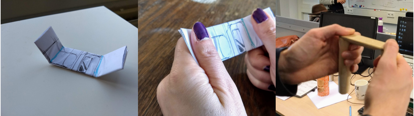
Figure 52. Different 3D models to test how users grab and hold the device.
