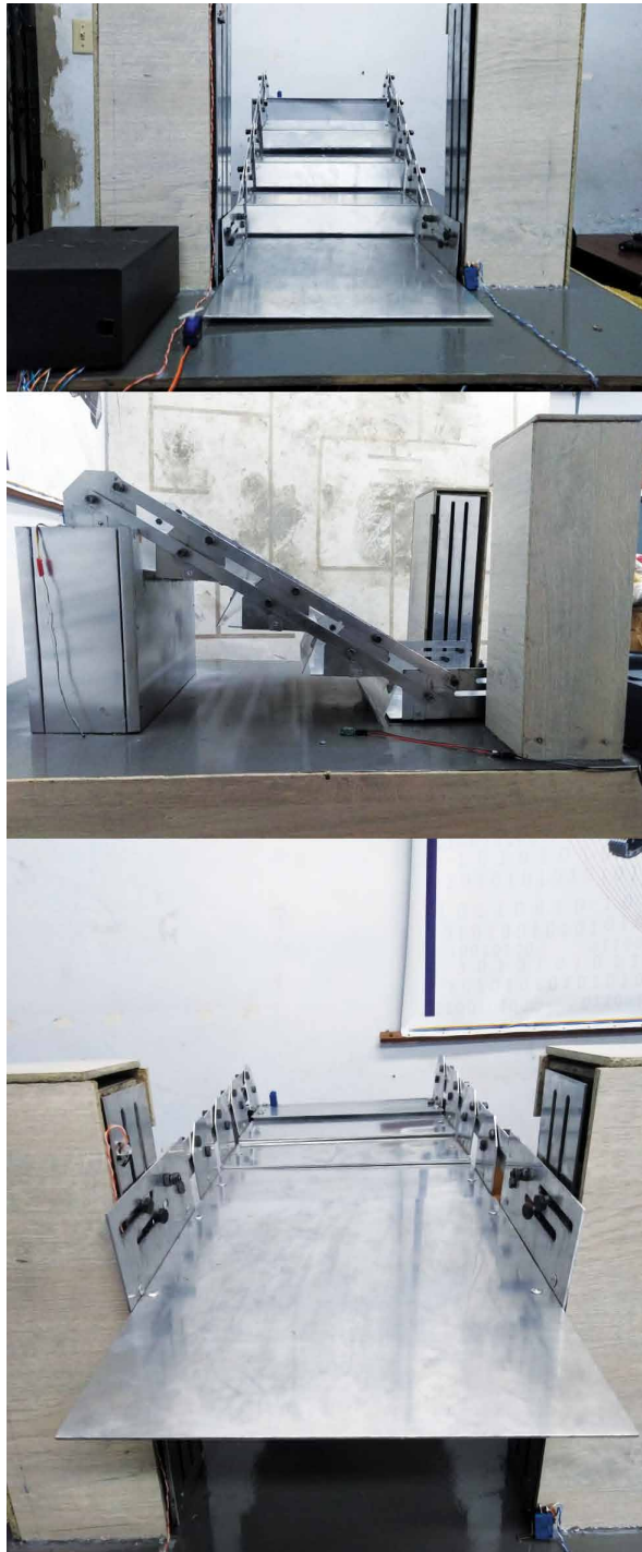
FIG. 5.42 Variation 2 configured for ( Top and Middle ) the 1st user-type (standard-stairs); and ( Bottom ) the 3rd user-type (elevating platform).
