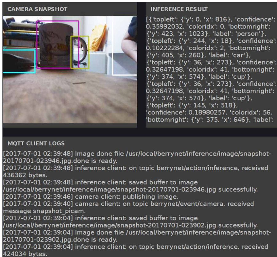
FIG. 5.11 Multiple-object detection via BerryNet®: 'person', 'cup'.
