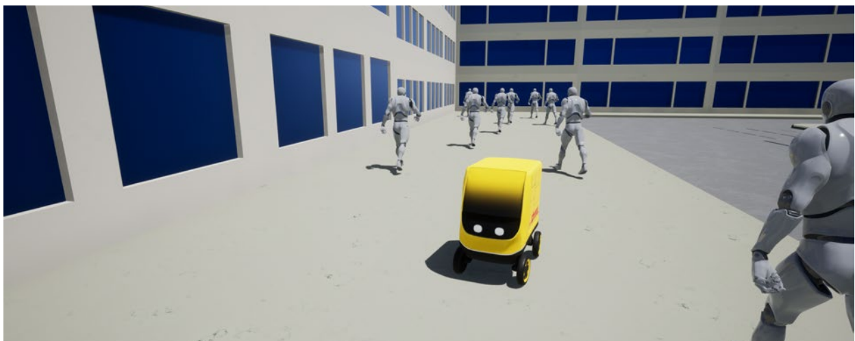
Figure 50. Scenario 2, in which the robot steers away from the pedestrian and the participant.
