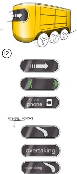
Figure 26. A display that shows an arrow when it is about to turn and a walking pedestrians animation if it will wait till everyone has passed.
