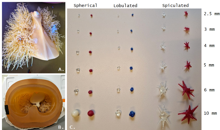
Figure 2.3: A. Artificial nodules situated in the lungs of the Lungman phantom, solid nodules were reflective with UV light. B. Lungs placed within the Lungman thorax. C. Overview of the artificial nodules, with different shapes, sizes and densities (Red/blue = subsolid -300 HU, White/Clear = solid +100 HU).
