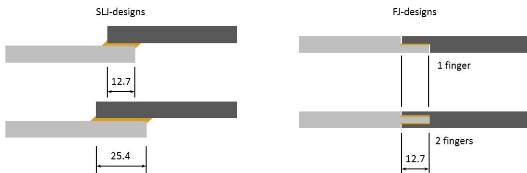
Figure 1: SLJ-designs and. FJ-designs tested.
