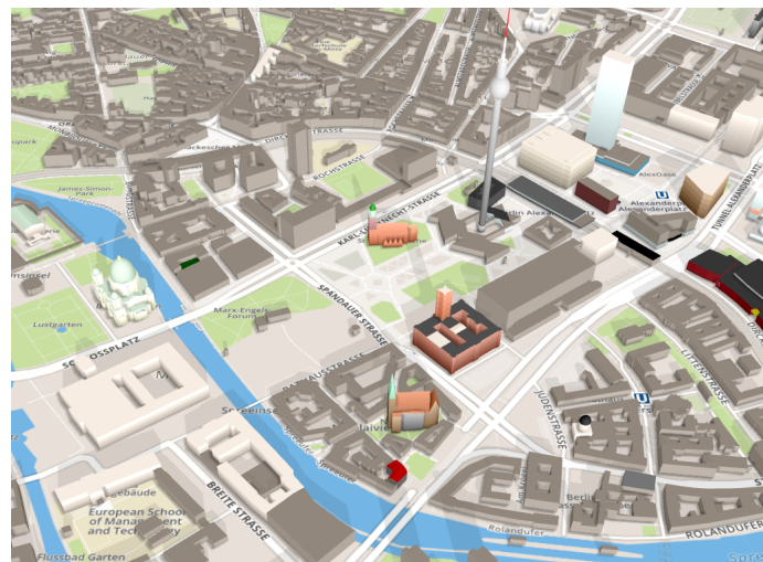
Figure 1.5: Landmarks are modelled in a higher LoD than the rest of the buildings in Berlin. Source: https://osmbuildings.org/
