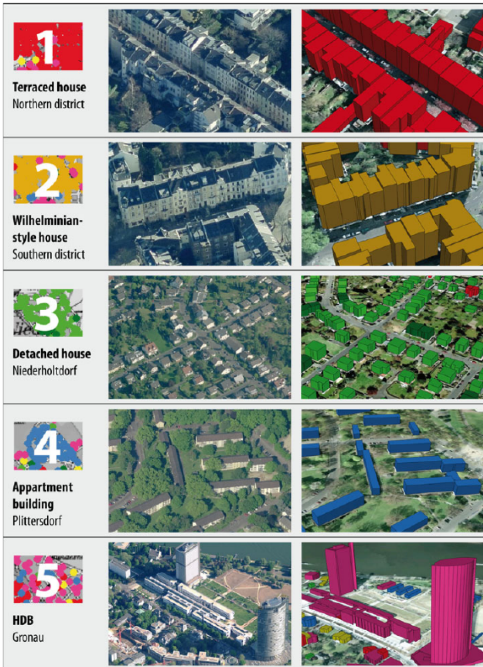
Figure A.1: Examples of building-type prediction in five exemplary districts of Bonn, Germany; source of left column: Microsoft Bing, of the aerial image in right column: Google Earth. Henn et al. [2012]
