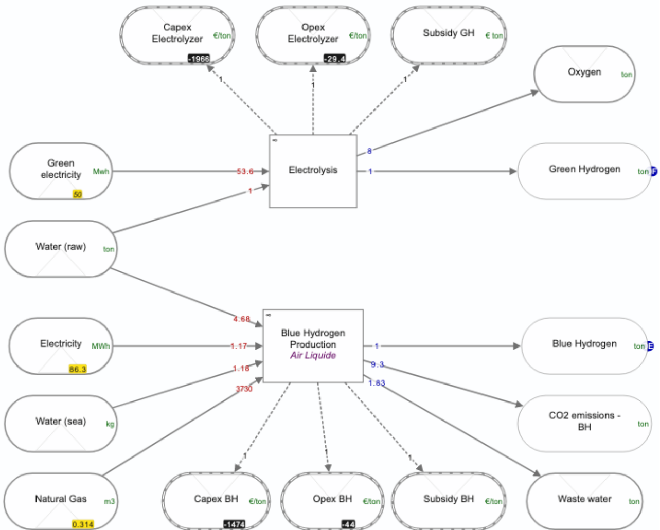
Figure 16: Linny-R model: Cluster of the domestic production of green hydrogen and blue hydrogen
