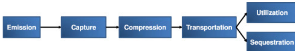
Figure 2: Simplified CCUS supply chain [10]
