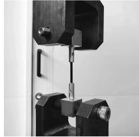
Fig. 7. Example of tubular joint specimen ( t_{out} = 2 mm) in the testing apparatus.
