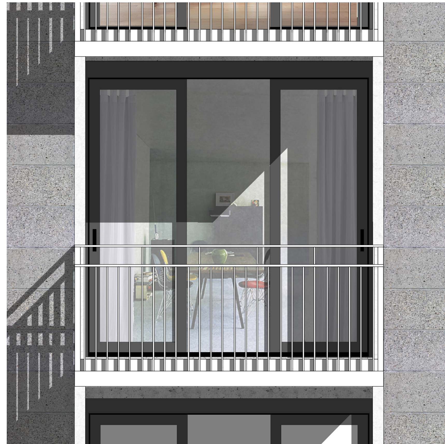
NEW BALCONY (2650 X 1600) Enlarged for functional use
