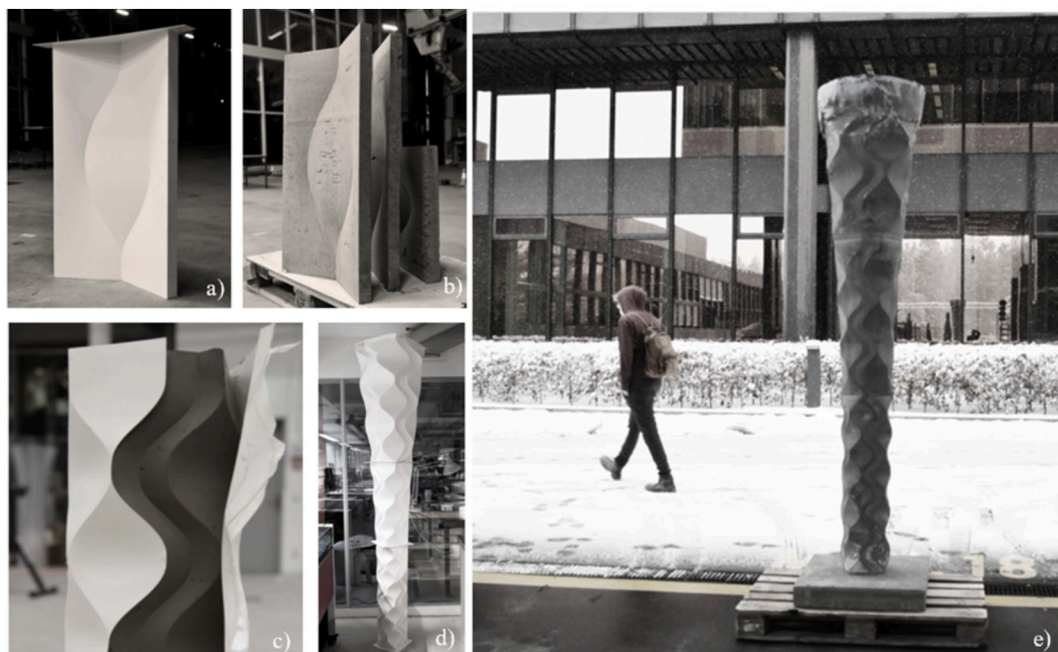
Fig. 23. a,b) Thin Folded elements [85], c) demoulding of first column, d) formwork for column, e) demoulded column produced with DCS [87].
