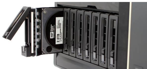
Figure 11.3: QNAP TS-879 Pro: an example with eight hot swappable hard drive bays. Received from Storage Review on 24 June 2015
