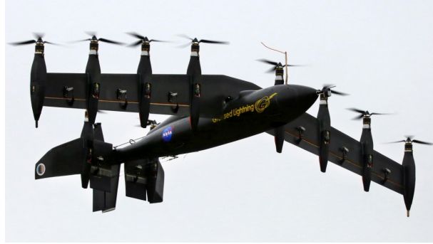
Figure 6.6: NASA GL-10 Greased Lightning: a tiltwing example.
