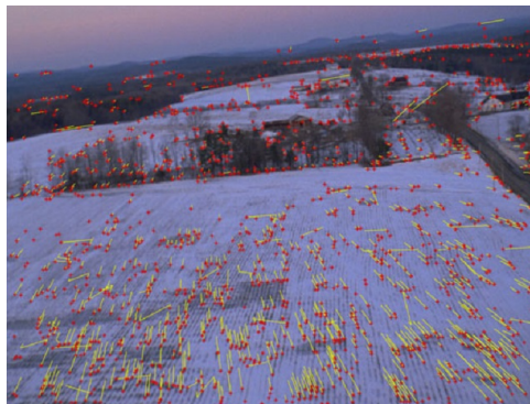
Figure 8.9: Sparse Optical Flow Example
