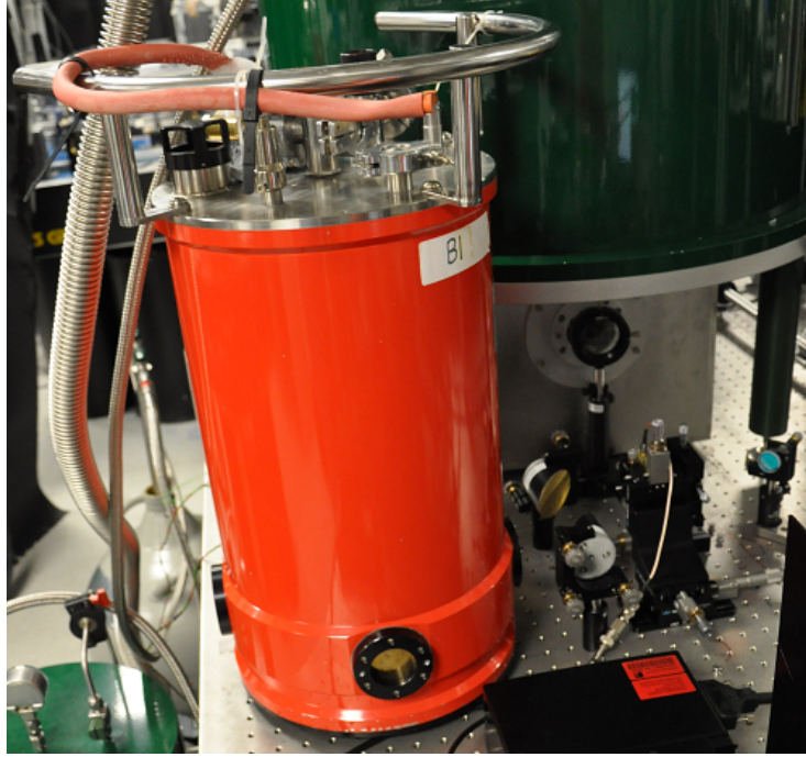
Figure 4.5: Measurement setup used for the alignment of the photoconductive antenna and the laser beam.
