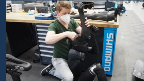
Figure 2.15: Some connection points are broken, so duct tape is used as an alternative.
