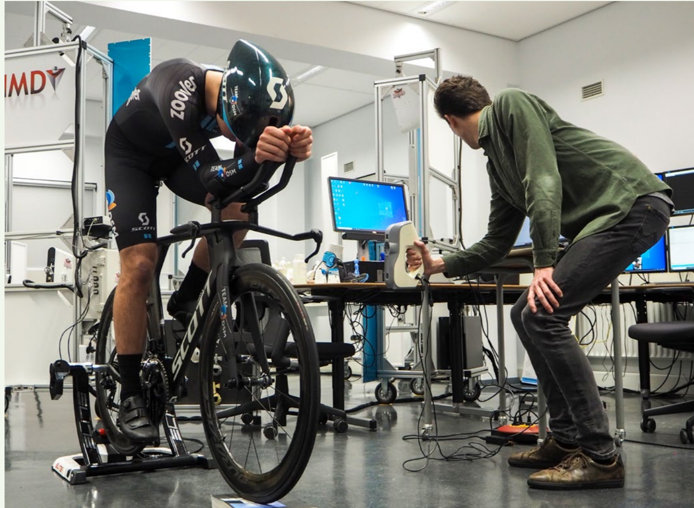
Figure 3.5: Capturing a participant in the Body Lab using a handheld 3D scanner.
