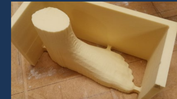
Figure 4.19: Milling is complete for the top side of the foot.
