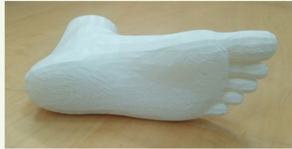
Figure 4.107: A rough surface remains after removing all supports.
