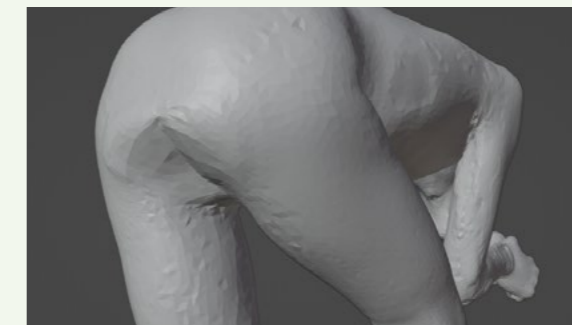
Figure 5.7: The bottom must leave enough space for any saddle.
