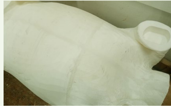
Figure 4.126: Filled seams after light sanding.
