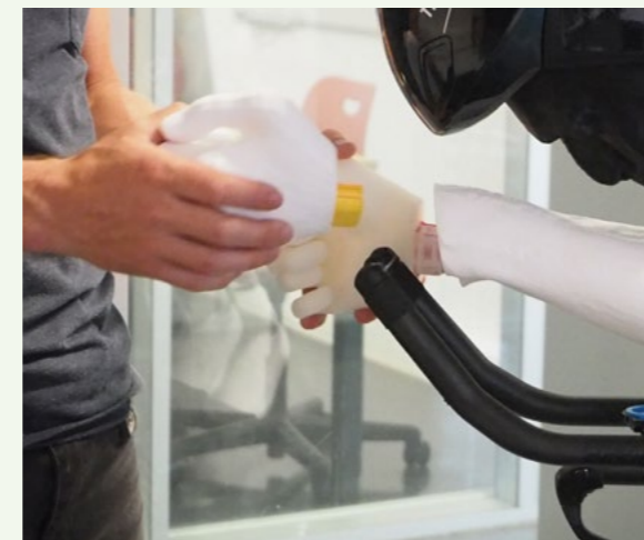
Figure 4.93: Flexible hands fold around the handlebar and attach to the arm.
