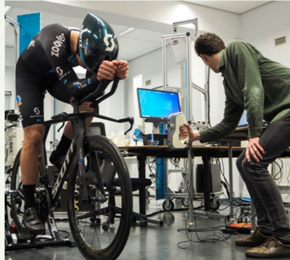
Figure 3.1: Capturing rider using 3D scanner.
