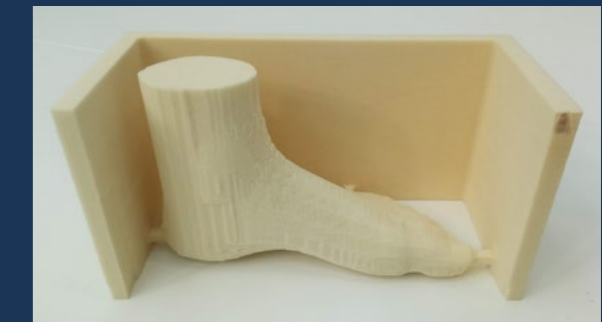
Figure 4.23: Result of the foot after CNC milling is completed.
