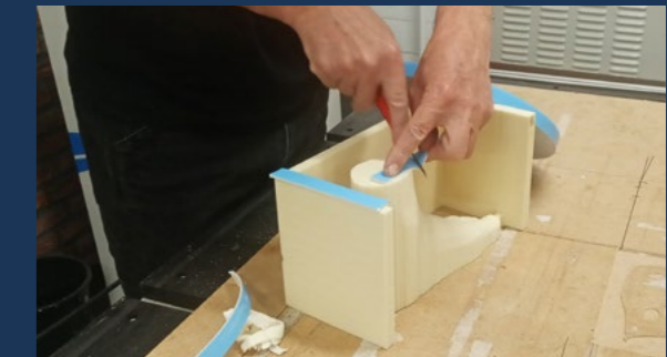
Figure 4.20: Double-sided tape is applied to the other side of the object.
