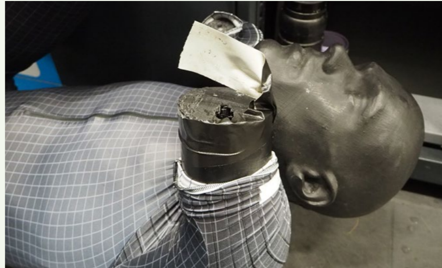
Figure 2.21: Elements connecting limbs have become too fragile and duct tape is used instead.
