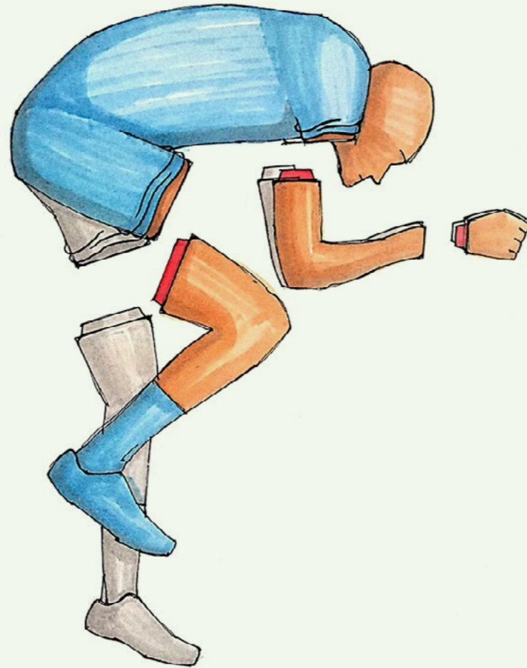
Figure 4.57: Segmentation of the mannequin in time trial pose.
