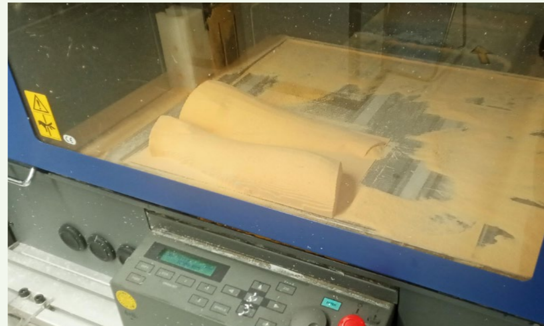
Figure 4.96: Two arm segments are CNC milled.
