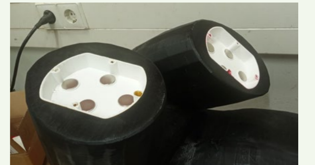
Figure 4.137: The interfaces are placed in the torso slots inverted to align them to the leg.
