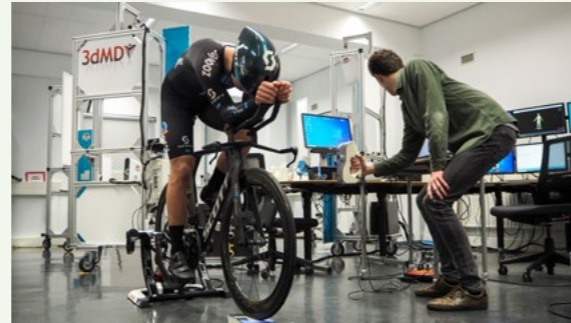
Figure 7.2: Participant positioned in time trial pose on the bicycle with a handheld scanner setup.
