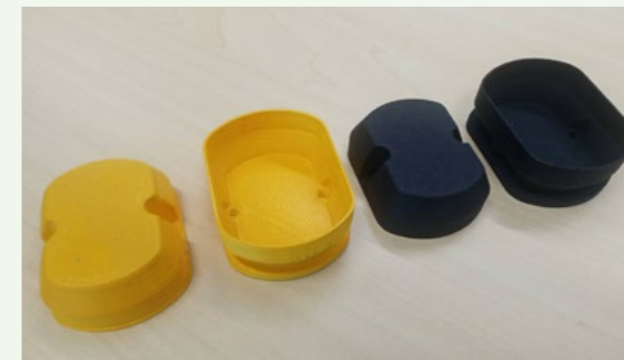
Figure 4.88: Sixth attachment interface FDM (yellow) and SLS 3D printed (black).
