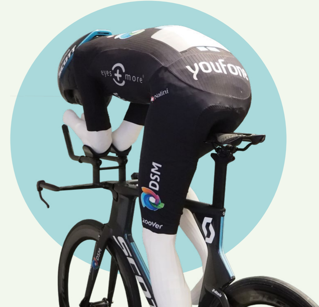
Figure 5.10: Personalized Mannequin of an individual male, professional cyclist in time trial pose.
