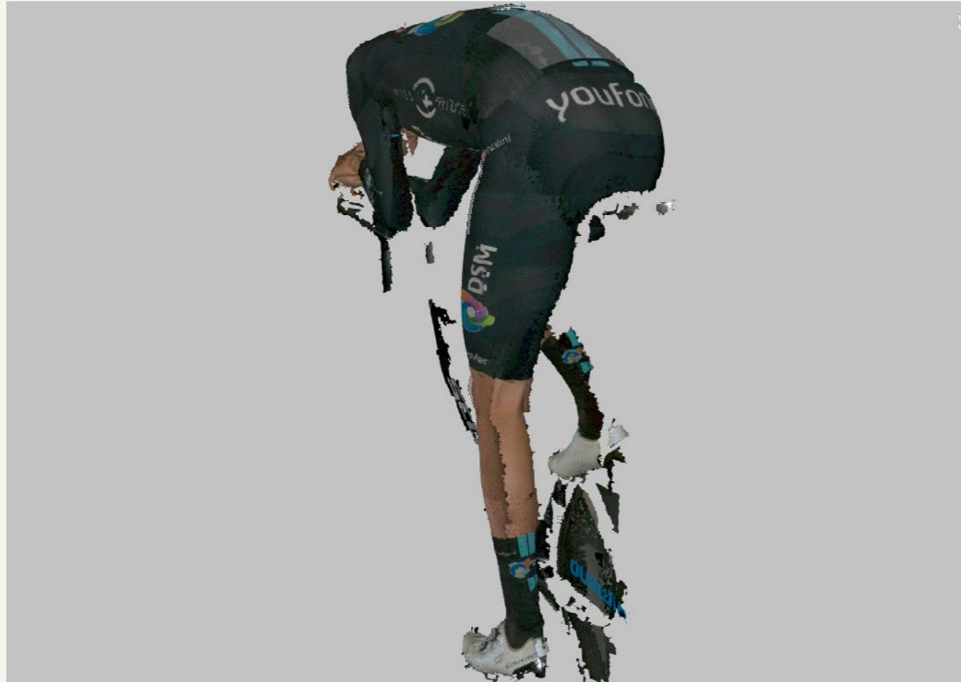
Figure 3.8: The raw scan data contains gaps and environmental elements.
