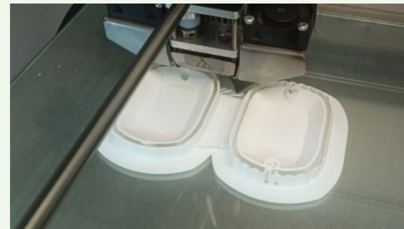
Figure 4.76: The object is FDM 3D printed layer by layer.
