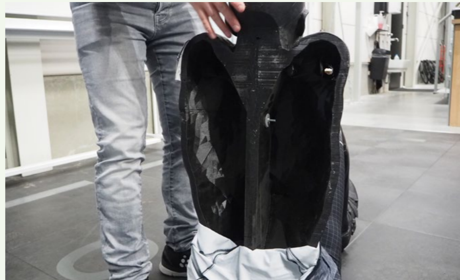
Figure 2.22: Limbs are connected to the torso using nuts and bolts, the back piece is attached last.
