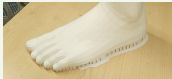
Figure 4.109: A left foot 3D printed vertically.
