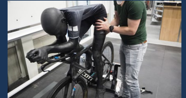
Figure 2.17: The legs are attached to the body, but do not actually connect to the pedals.
