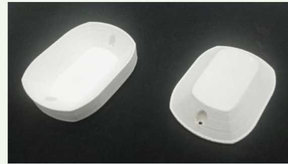
Figure 4.77: After removing the brim and support, the result needs little finish.
