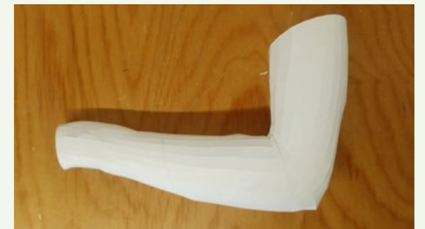
Figure 4.105: Upper, middle and lower arm segments glued together.
