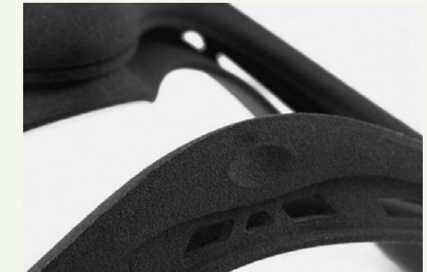
Figure 4.39: FormLabs. (n.d.). [Photograph of SLS parts showing a grainy surface, but are easy to finish].
