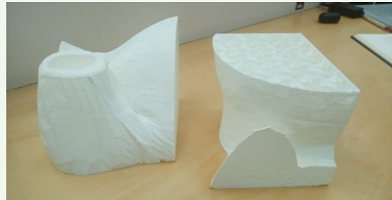
Figure 4.121: First torso segments suffer from surface errors.
