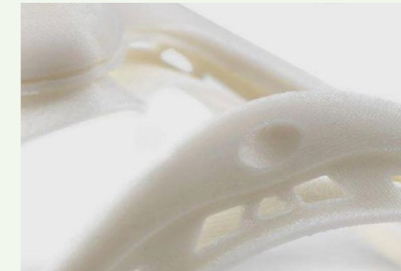
Figure 4.37: FormLabs. (n.d.). [Photograph of FDM parts showing layer lines and inaccuracies in the surface].
