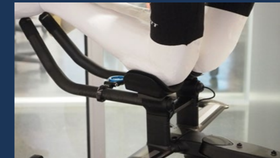
Figure 4.7: The arms are placed on the elbow rests and the hands on the bar-ends.
