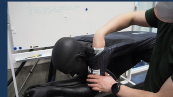
Figure 2.18: Limbs are manually secured to the torso with integrated nuts and bolts.
