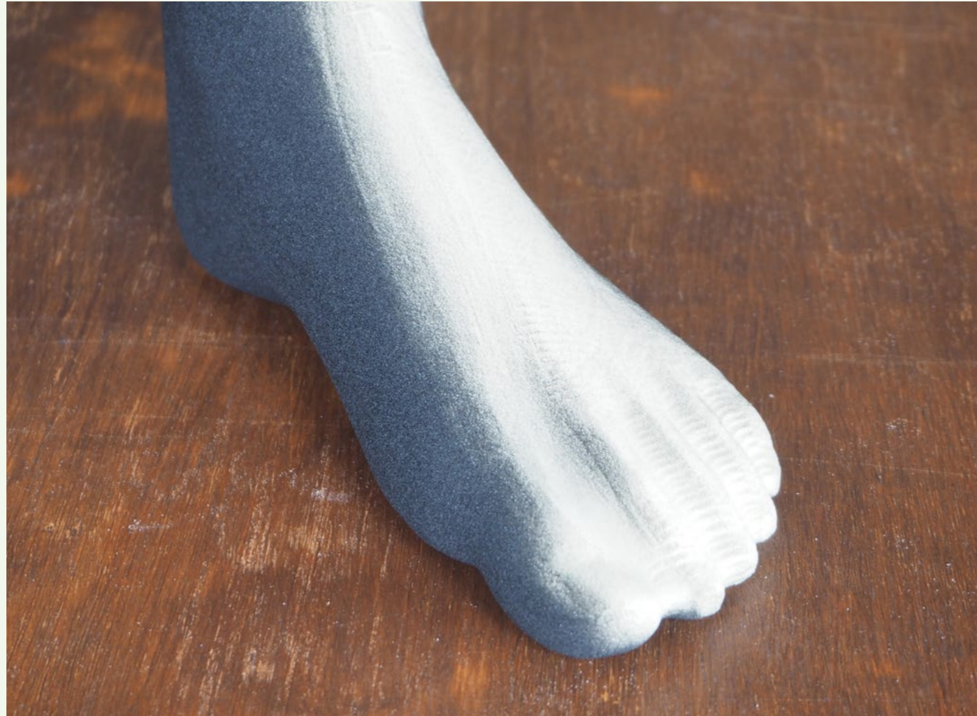
Figure 4.24: A partially sanded and coated, CNC milled foot prototype.
