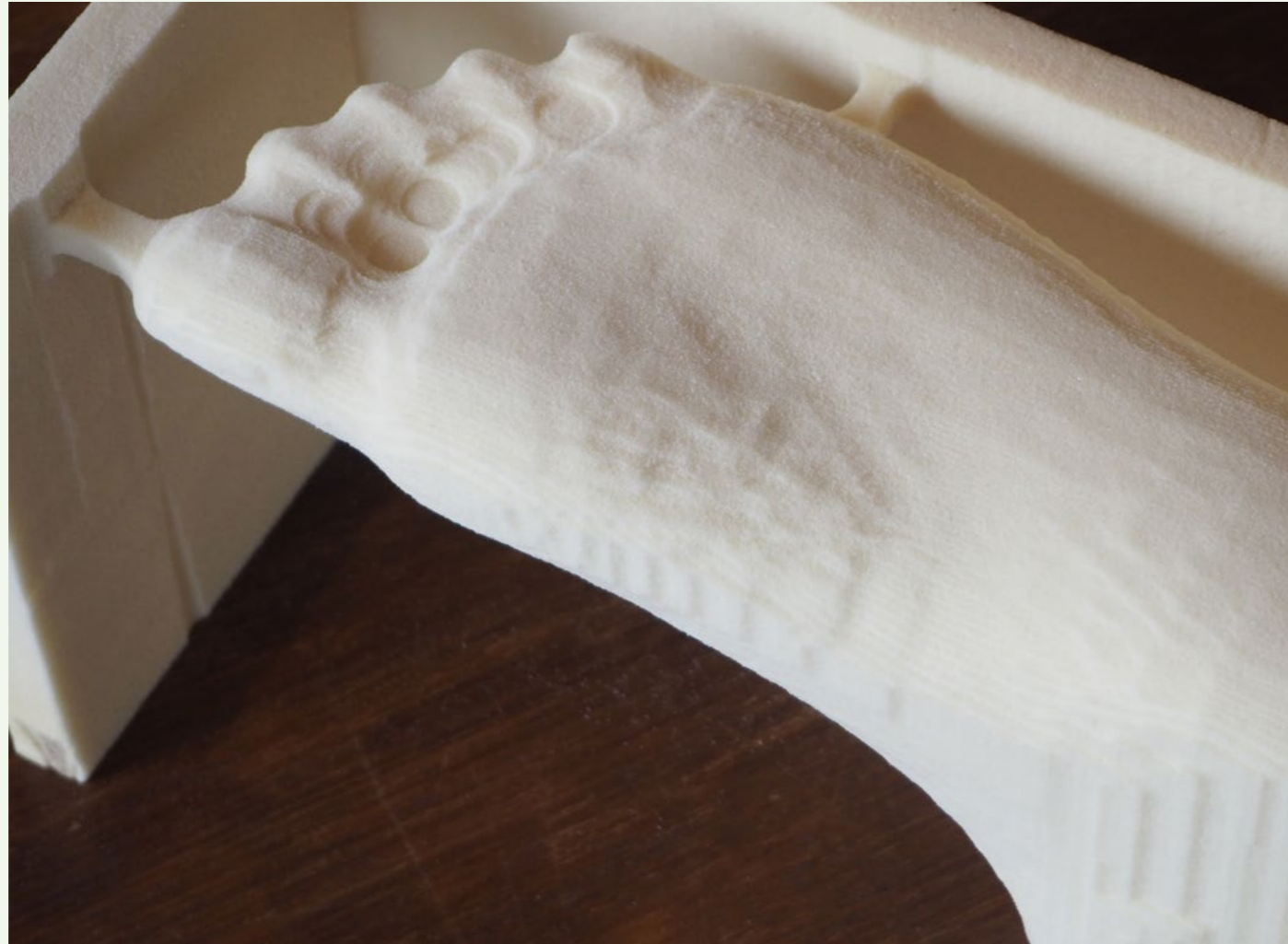
Figure 4.15: An untreated, CNC milled foot prototype with box supports.
