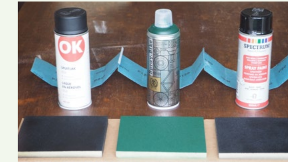
Figure 4.26: The resulting foam tiles after coating.
