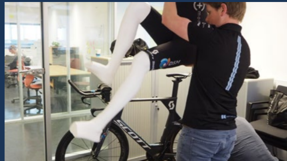
Figure 4.147: The assembled mannequin has to be lifted over the bicycle.
