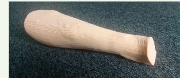
Figure 4.100: Milling marks on the arm segment.
