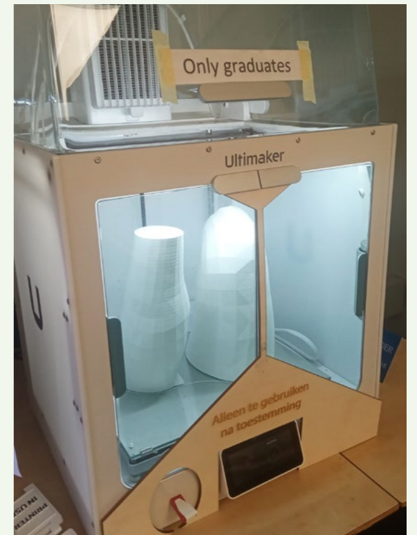
Figure 4.119: An upper and lower leg segment completed by the Ultimaker S5.
