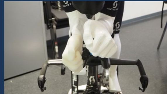
Figure 4.148: The arms are asymmetric and the hands do not connect with the bar-ends.
