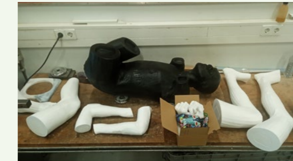
Figure 4.135: All separate parts of the mannequin to assemble.
