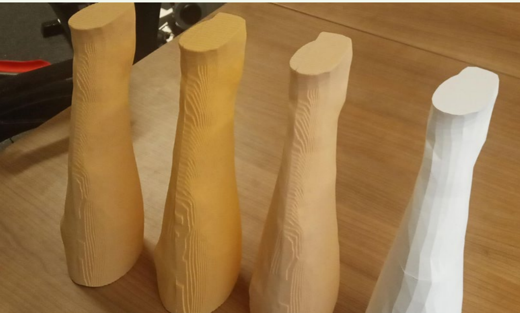
Figure 4.95: Three CNC milled and one 3D printed lower arm segments.
