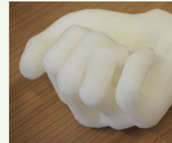
Figure 4.95: A hand made of flexible TPU.
