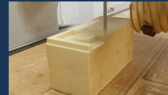
Figure 4.18: The first layer is CNC milled and frame contours become visible.
