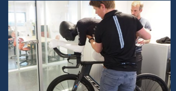
Figure 4.6: The assembled mannequin is placed on the bicycle in a stand.
