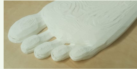
Figure 4.108: Holes appear near flat sections because of the layer height setting.
