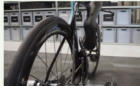
Figure 2.6: The Dumoulin Mannequin's feet are not easily attached to the pedals.
