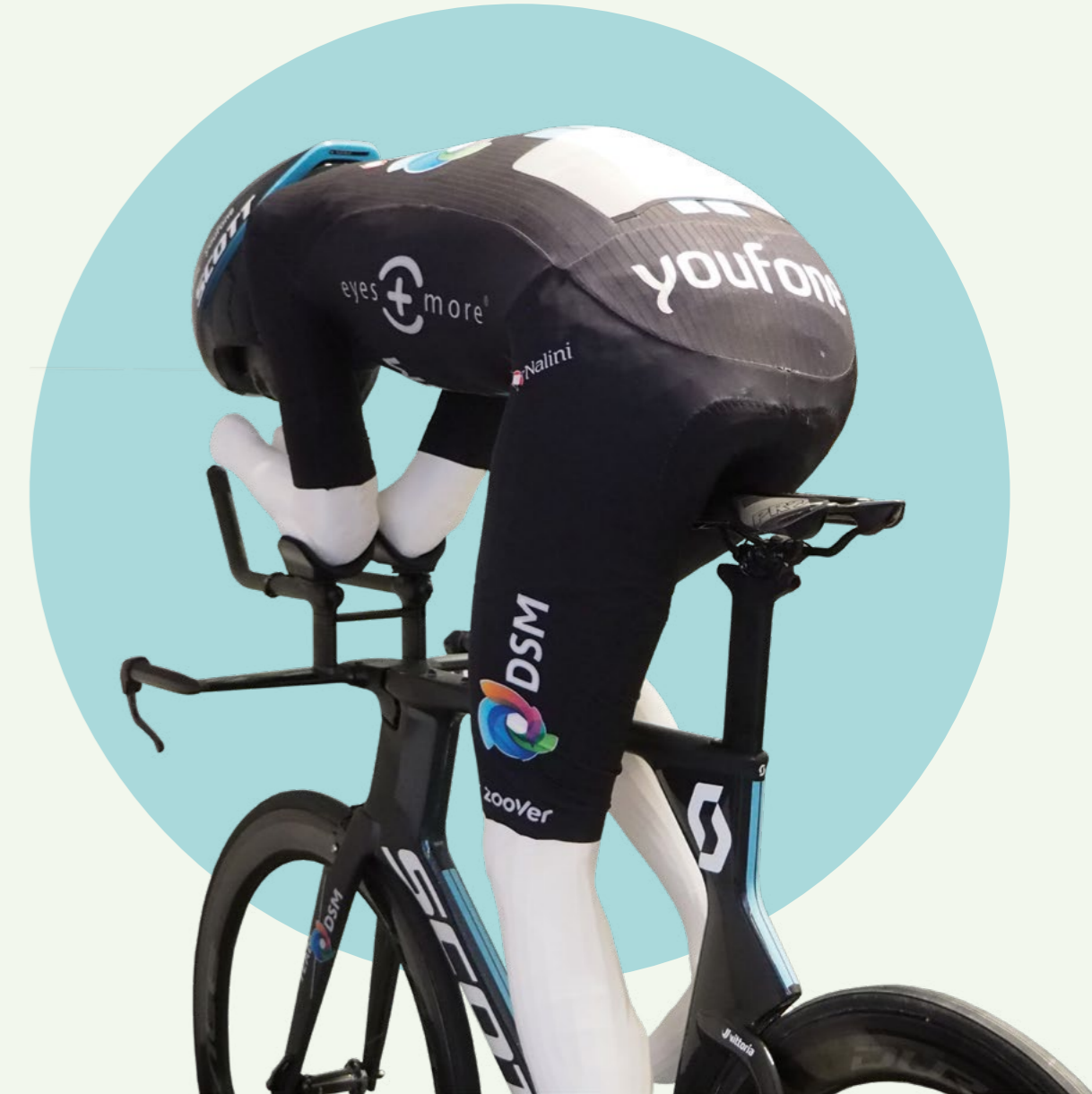
Figure 0.2: Personalized Mannequin of an individual male, professional cyclist in time trial pose.
