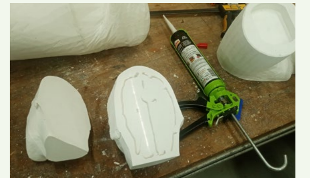
Figure 4.124: Applying kit to one of the surfaces.
