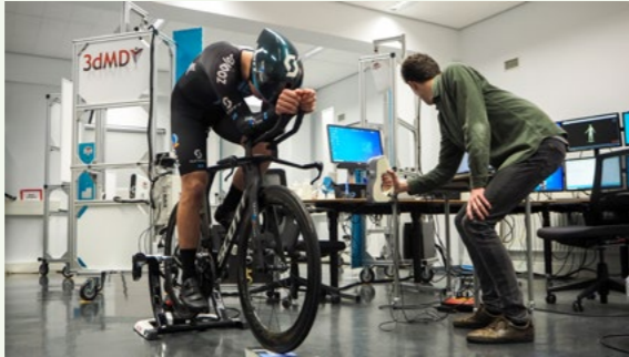
Figure 7.11: 3D Scanning a participant on a TT bicycle.
