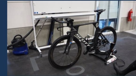
Figure 2.13: The bicycle is easily installed in a fixed stand.
