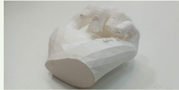
Figure 4.106: Remains of the supports are clearly visible near the fingers.
