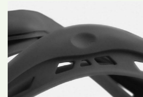
Figure 4.38: FormLabs. (n.d.). [Photograph of SLA parts showing a smooth surface that requires little finishing].
