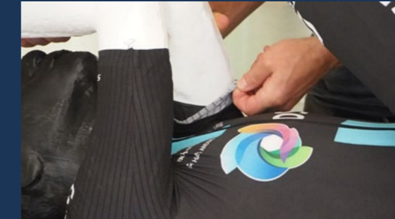
Figure 4.5: The sleeves of the cycling suit cover the seam between the limbs.
