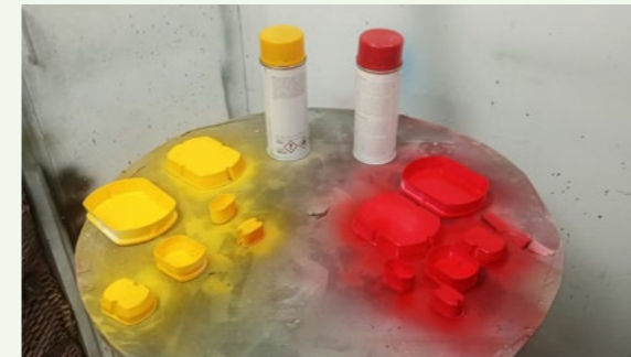
Figure 4.134: The attachment interfaces after applying a layer of paint.
