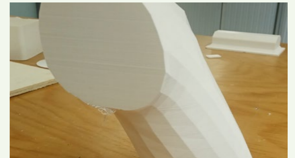
Figure 4.104: A small failure in the upper arm where support is required.
