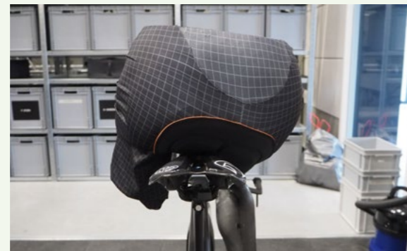
Figure 2.5: The Dumoulin Mannequin has a small contact area with the saddle.
