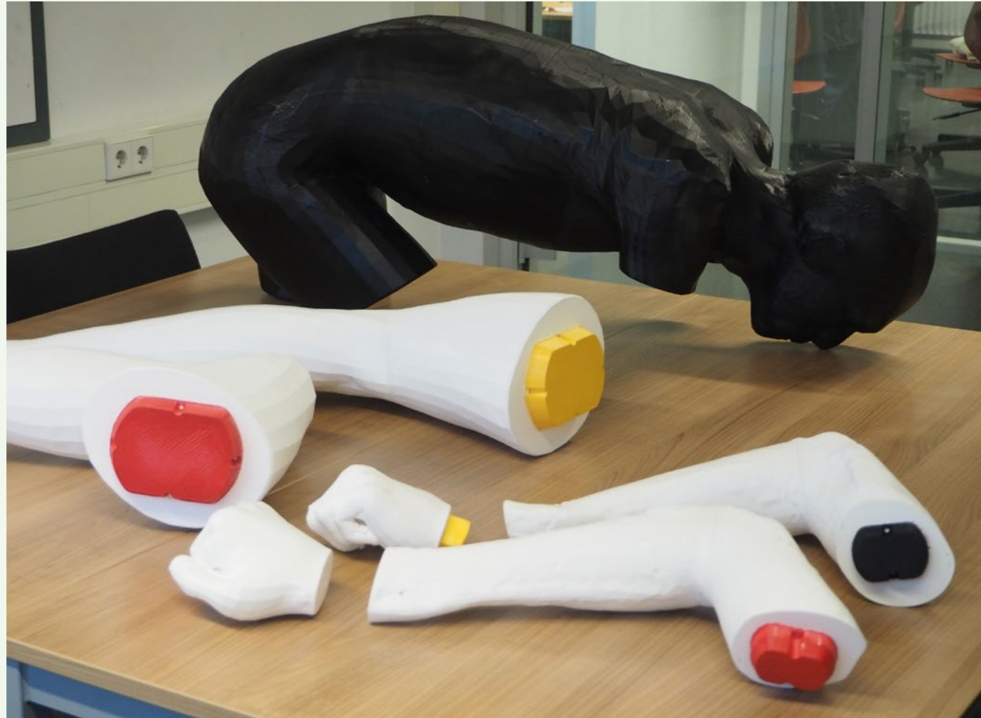
Figure 4.67: Design of the arm attachment interface on various limbs.
