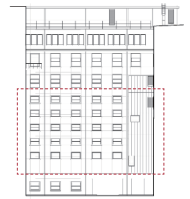
Inner Elevation of Block XVI Low ceiling Height: 2.5 m
