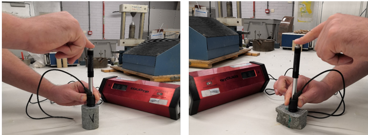
Figure 5.1: Left is the Equotip test on a drill core. Right is Equotip test on a cut block
