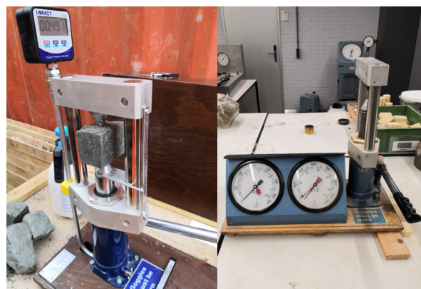
Figure 5.4: Left: Impact Digital Point Load Test equipment used at the mine. Right: ELE Analogue Point Load Test equipment used at the TU Delft
