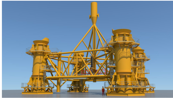
Figure 1.2: Pile installation frame for Beatrice OWF (with worker mid-right)
