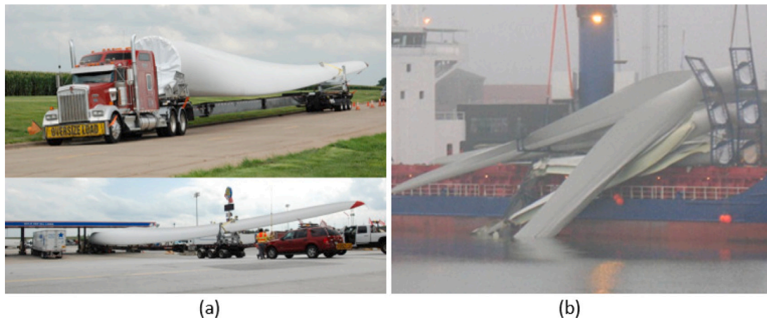
Fig. 6. (a) Onshore transportation of blade (permission taken from Elsevier [48]) (b) Blade damage during offshore transportation (permission taken from Skuld [49]).
