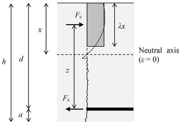
Figure 8. Calculation of moment resistance capacity.
