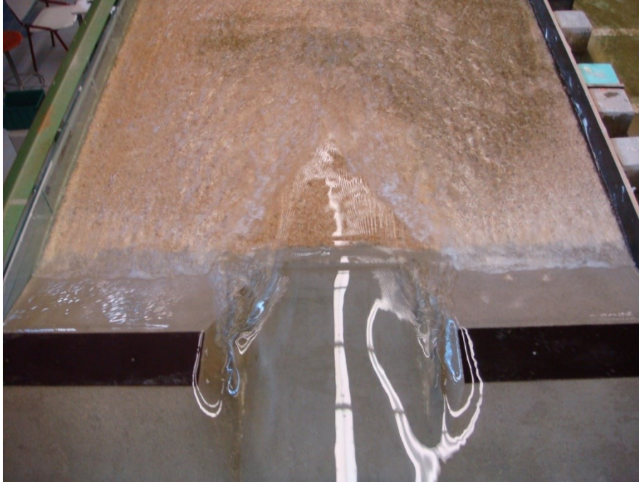
Figure 3.20 Breach flow pattern in compound weir condition ( Q = 50 l/s, case 5)
