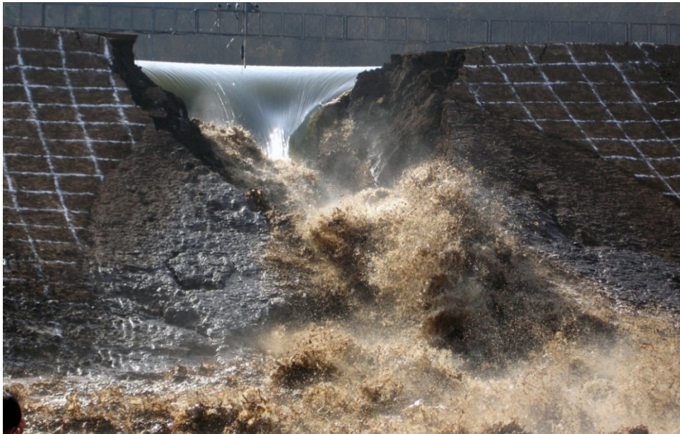
Figure 2.9 Earthen dam breach test in Nanjing Hydraulic Research Institute (Zhang, et al. , 2009)
