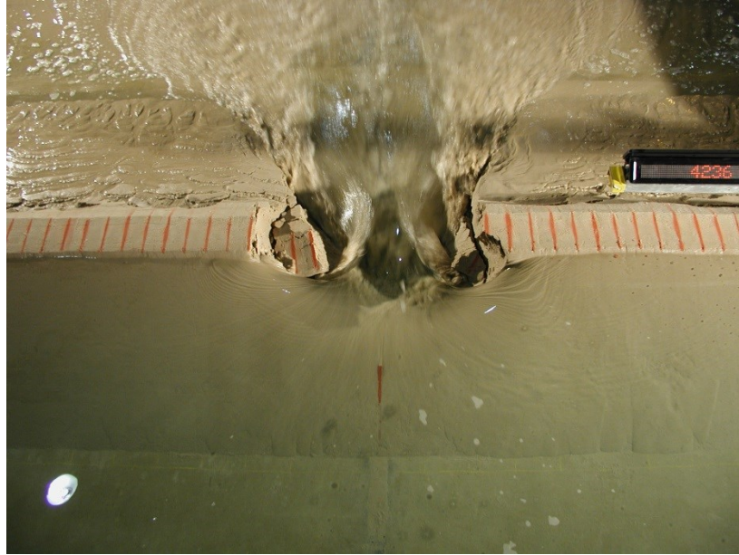
Figure 2.7 Breach of sandy dike in HR Wallingford (Test 2)
