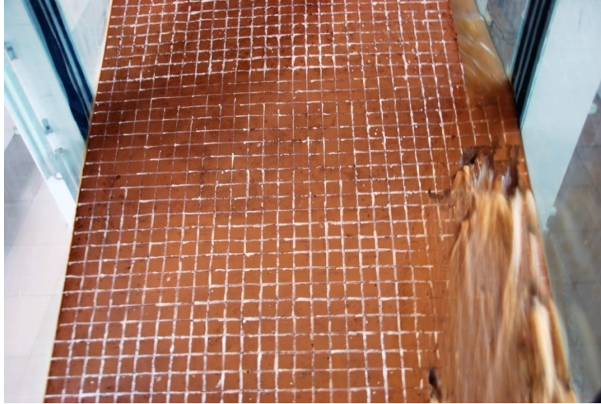
Figure 5.26 Surface erosion at the initial phase of breach (Run 4)
