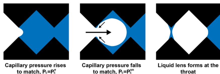
Figure 13: Conditions for Roof snap-off illustrated. Based on Rossen (2003)
