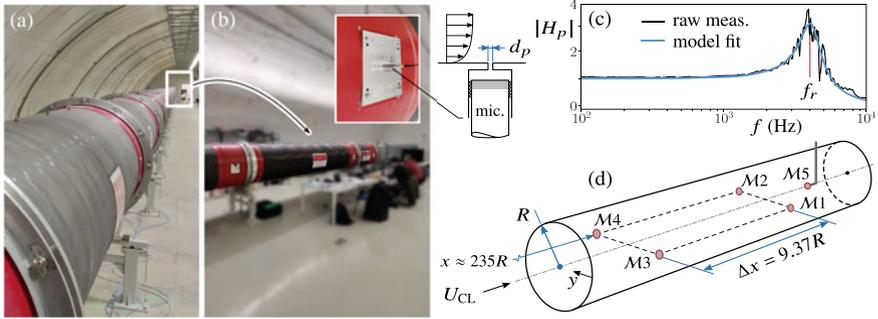
**Fig. 1** **a, b** Photographs of the CICLoPE facility and test section; **b** one of the four wall plugs with the microphone sensor; **c** gain of the transfer function between inlet and cavity pressures, measured in quiescent flow; **d** microphone lay-out with  $x = 0$  corresponding to the pipe inlet
