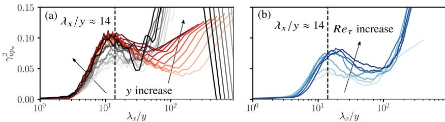
**Fig. 3** **a** Coherence spectra of wall-pressure and streamwise velocity in the logarithmic region for DNS channel flow data (red, [12]) and experimental data (black, [11]) at  $Re_\tau \approx 2\,000$  and for 10 logarithmically spaced locations in the range  $y^+ \in (80, 200)$ . **b** Coherence spectra of wall-pressure and velocity for data acquired in the CICLoPE facility
