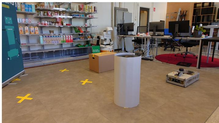
**Figure 5.16:** Setup for the real-world experiment in the retail store environment lab of AIRLab Delft [1], showing the ground robot to the right and two random obstacles in the middle.
