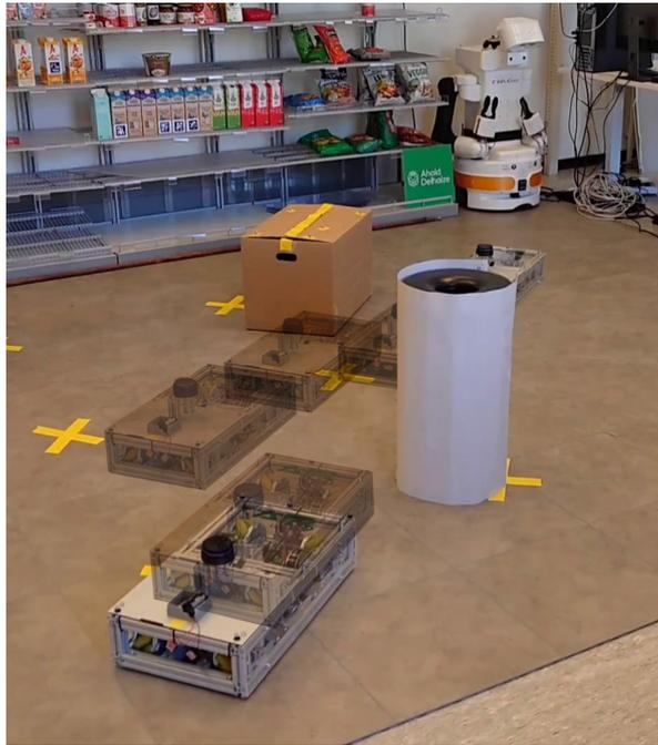
**Figure 5.17:** Motion of the robot during the real-world experiment in an environment with two obstacles. The robot's initial location is shown at the bottom, while the goal location is positioned at the top right.
