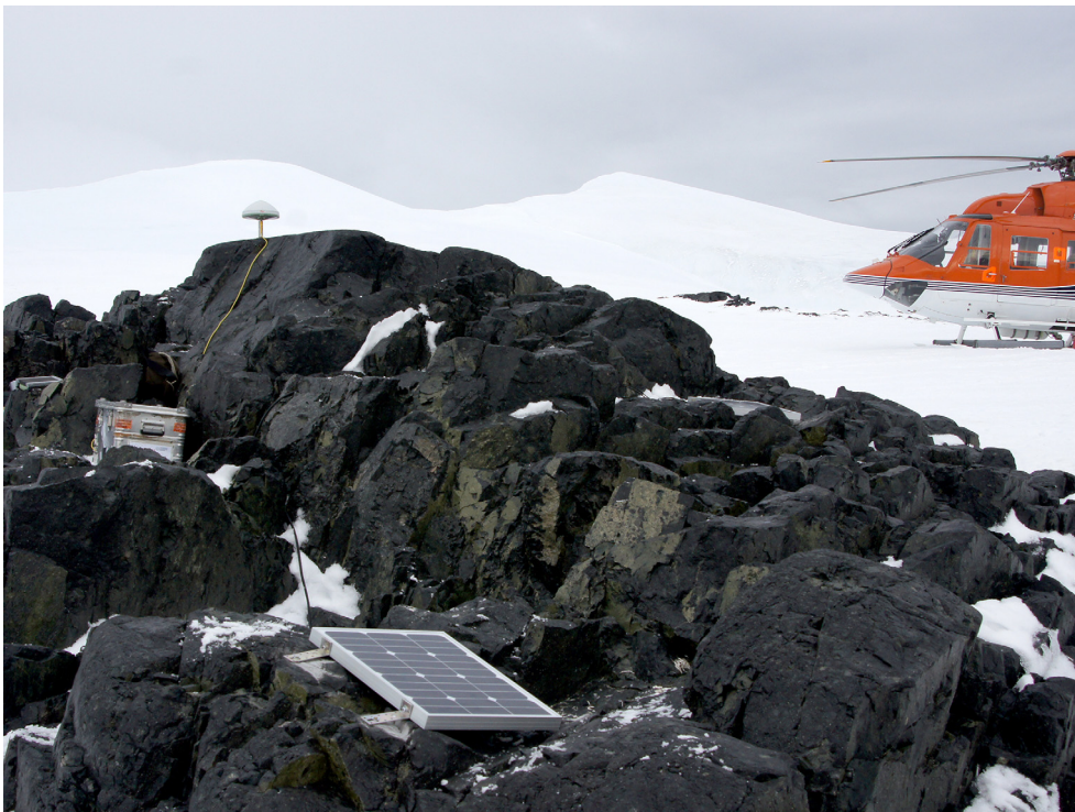
Fig. 1. Example of a GNSS campaign site: Clark Island, Pine Island Bay, West Antarctica. The GNSS antenna is fixed to the bedrock. Receiver, battery and electronics are stowed in an aluminium box, while the solar panel is used to recharge the battery. Image credits: M. Scheinert.
