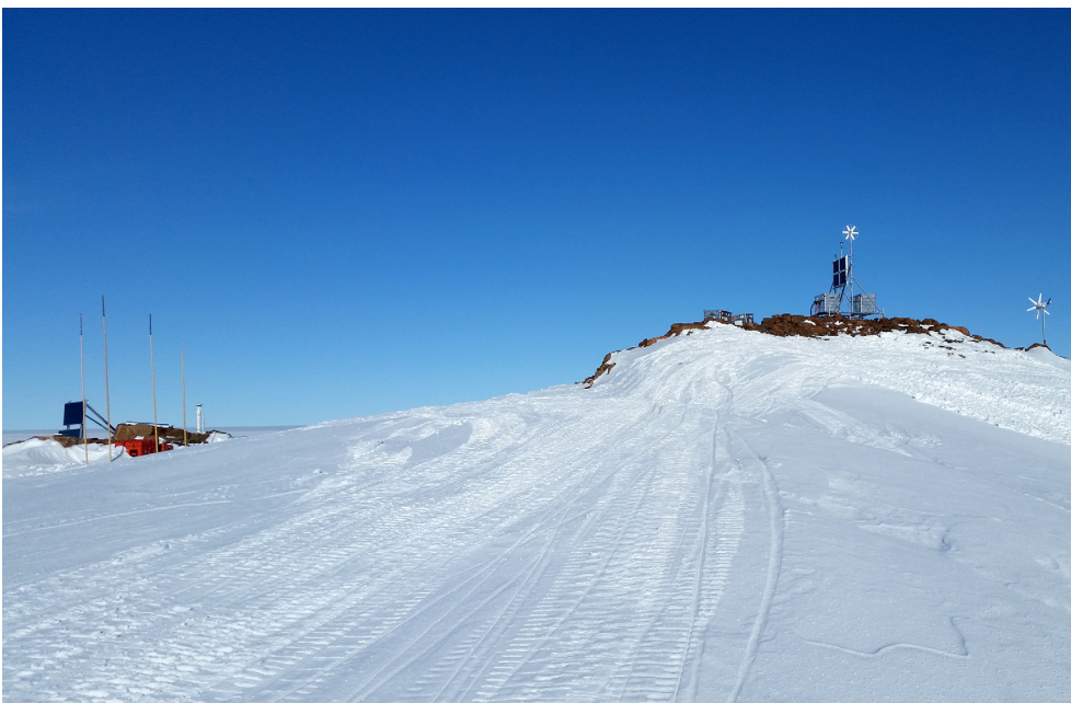
Fig. 3. Example of a GNSS permanent site: Kottas Mountains, western Dronning Maud Land, East Antarctica. The GNSS antenna is installed on the left outcrop (see also Fig. 4). This GNSS site is co-located with a seismometer station of the Alfred Wegener Institute, Germany. On the right outcrop, solar panels and wind generators are mounted. Image credits: E. Buchta.
