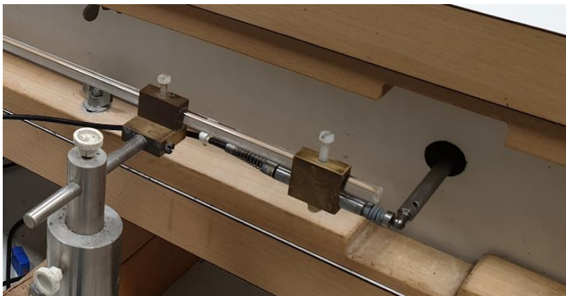
figure F.5 LVDT's and embedded bars of ADTM test
