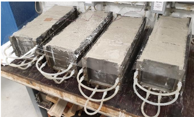
figure F.8 Cubes in the temperature regulating moulds
