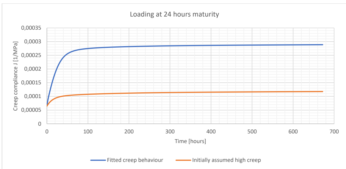
figure G.2 Comparison between the total strain response to unit of stress according to the fitted creep behaviour and the initially high creep behaviour for a maturity at loading of 24 hours
