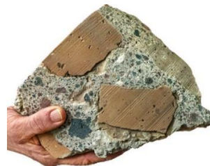
figure 1 Colosseum, Rome. Example of durable roman concrete (Smithsonian, 2011; The American society of mechanical engineers, 2017)
