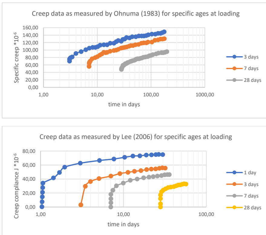
figure 49 Examples of results of creep measurements on young concrete (Bažant et al., 2014).
