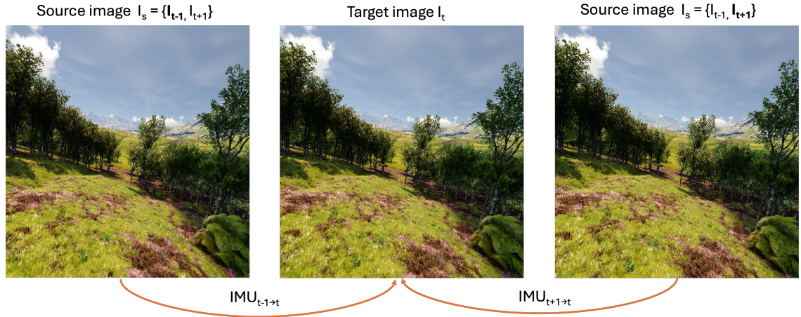
Figure 3.2: Input snippet for the model, consisting of two source images, a target image, and IMU data between consecutive frames.
