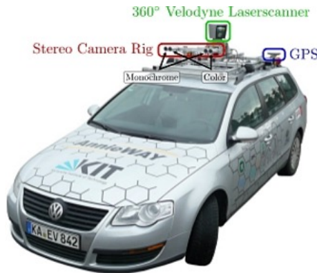
Figure 1.5: The vehicle used for capturing the KITTI dataset, equipped with high-resolution stereo cameras, a laser scanner, and precise GPS/IMU navigation systems for data collection in autonomous driving scenarios.
