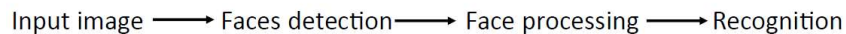
Figure 2.6: Pipeline of a facial expression recognition algorithm. First faces are detected from the input image. Then they are processed and fed into the recognition algorithm.
