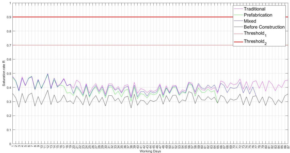
Figure 4.6: Average daily saturation rate R over the lifetime (working days) of the construction project for 3 different scenarios
