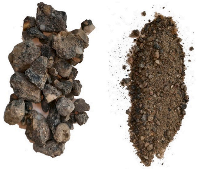
Fig. 5. Two fractions produced by traditional recycling: coarse recycled aggregate (>4 mm; left) and fine recycled aggregate (0–4 mm; right).
