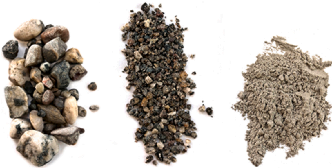
Fig. 6. Innovative recycling produces at least three fractions: secondary gravel (left), secondary sand (middle) and residual cementitious fines (right).
