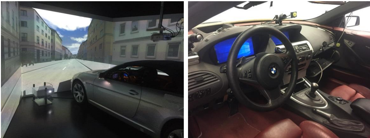
Figure 1. The TU Munich Driving Simulator. Left: full-vehicle mock-up; Right: cabin.
