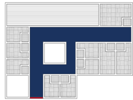
Nursing Home Groningen 3 1 Locked Entrance Long Hallway multiple direction possibility to wander
