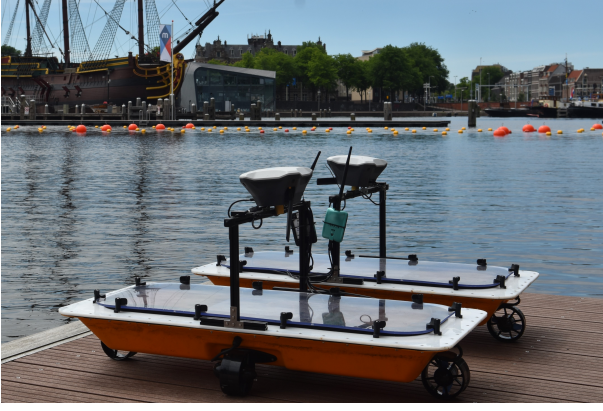
Fig. 1: 1:4 scale Roboat units on the quay in Amsterdam
