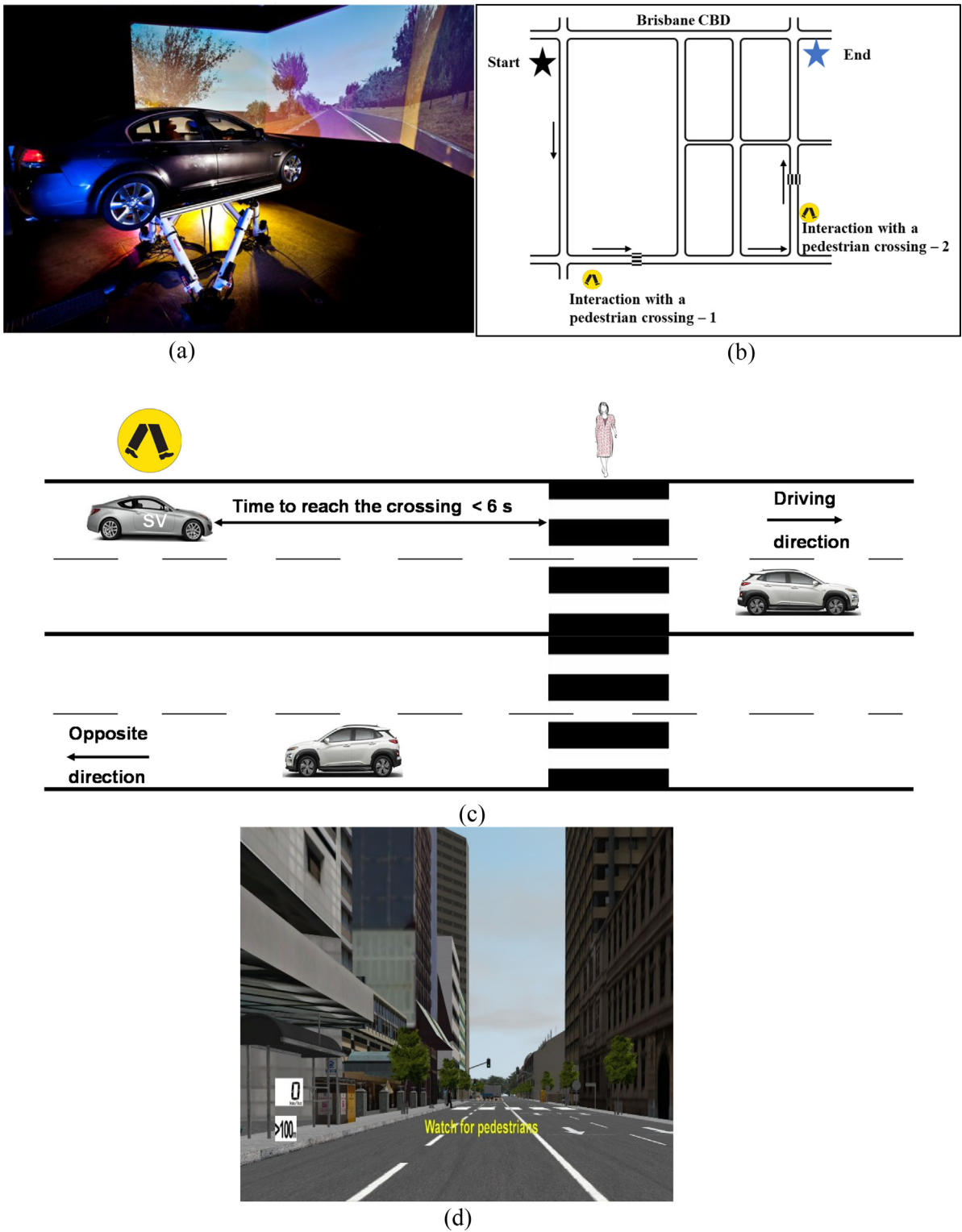
Fig. 1. Experiment design: (a) Advanced Driving Simulator; (b) Schematic of Brisbane Central Business District; (c) Designed vehicle–pedestrian interaction; (d) Design of advance information driving aid.
