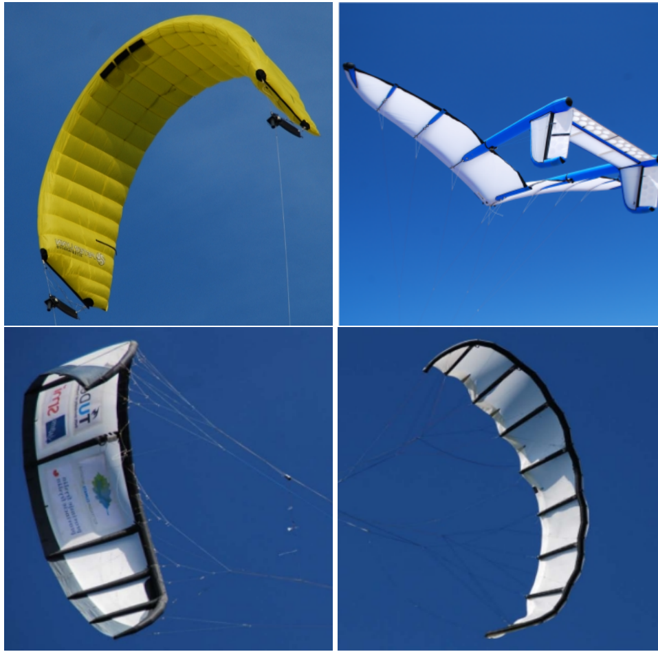
Figure 1.1: Different TU Delft concepts, top left: Ram-air, top right: kiteplane, bottom left: LEI (V2), bottom right: LEI (V3) [18]
