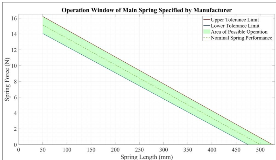
Figure 29: Operation window of Main Spring [85].
