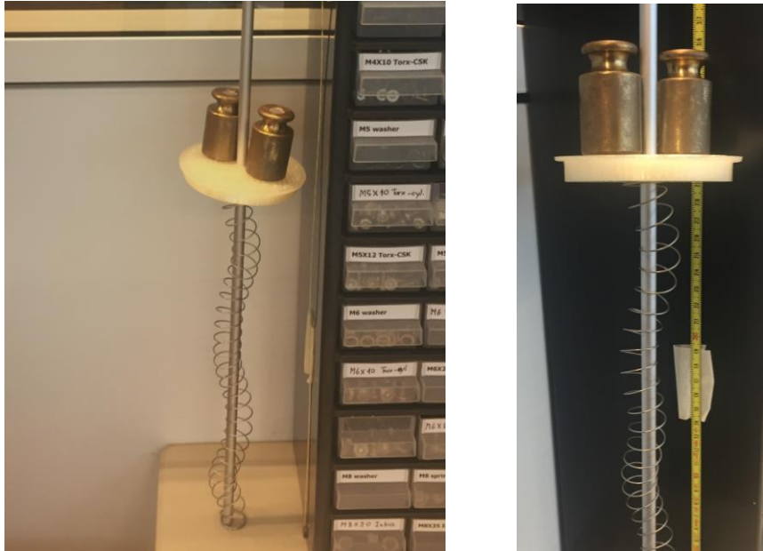
Figure 117: Main Spring Characterization Test Setup.
