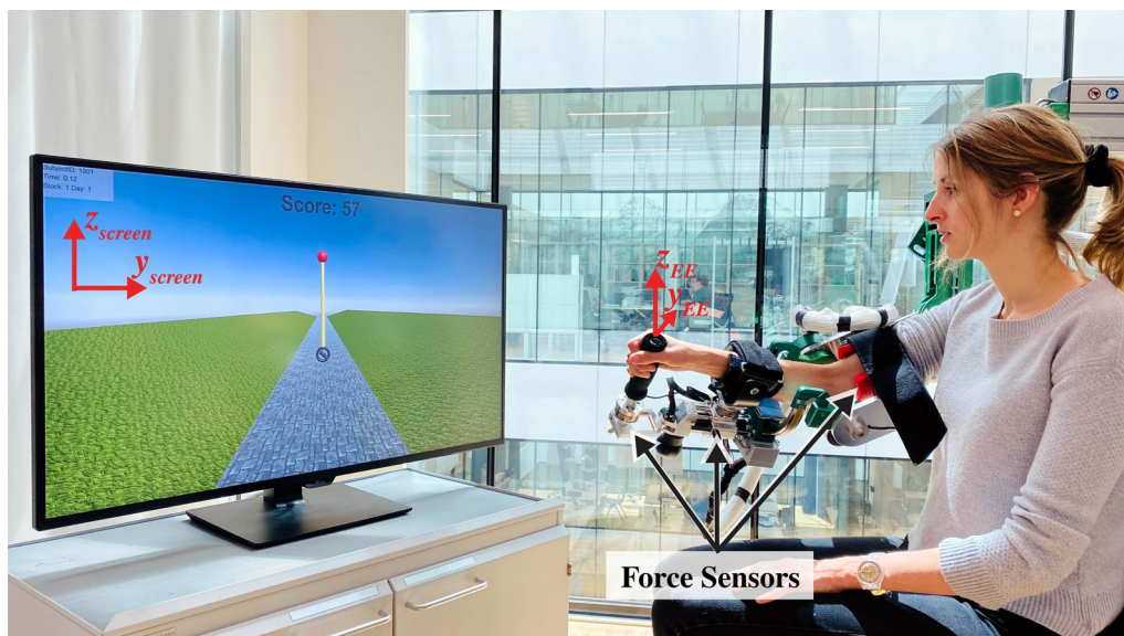
Fig. 1 Experimental setup with the ARMin exoskeleton robot. The motor task consisted of inverting a pendulum and keeping it inverted. The pivot point of the pendulum was matched to the movement of the hand module of the robot. The force/torque sensors below the lower/upper arm cuffs and below the hand module allowed participants to move the robot transparently through the use of disturbance observers
