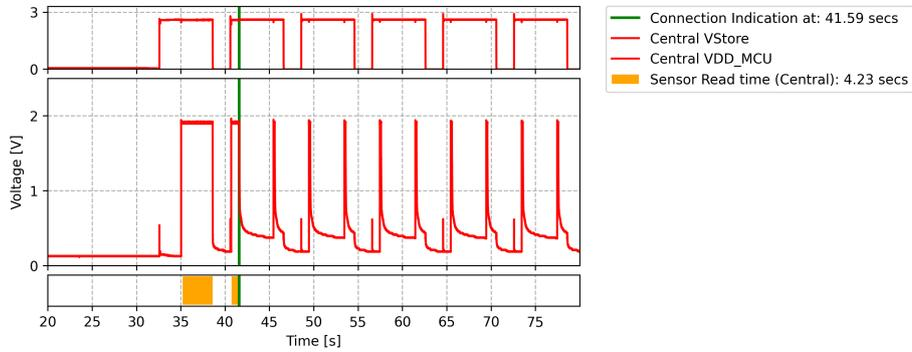
(b) Voltage measurement for central device
