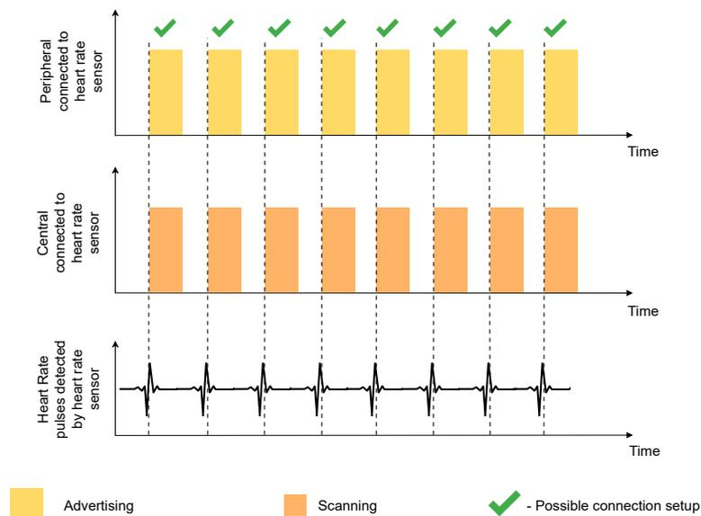
(b) Successful synchronised connection setup attempts in a CardioSync system. Advertising of peripheral and scanning of central is synchronised by heart rate pulses detected by heart rate sensor connected to the devices.
