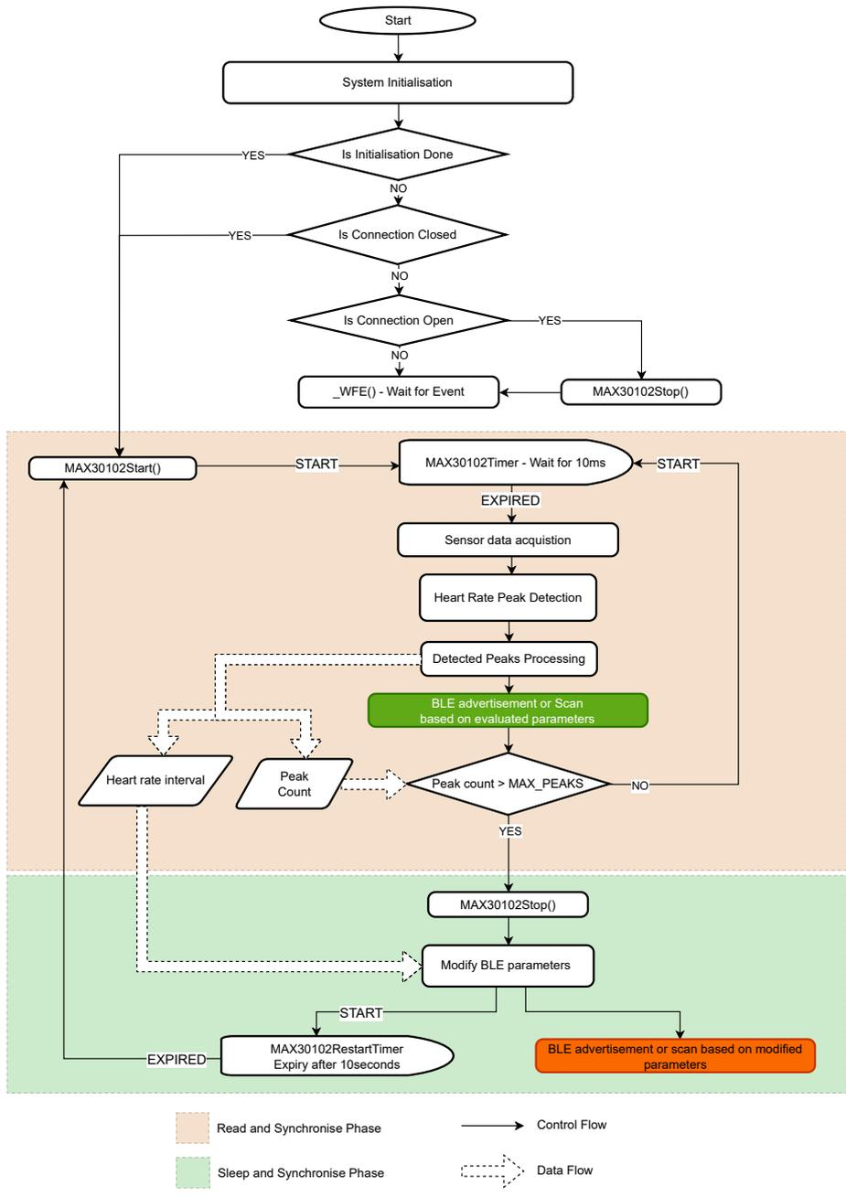
Figure 4.4: Operation flowchart of the CardioSync framework implementation.
