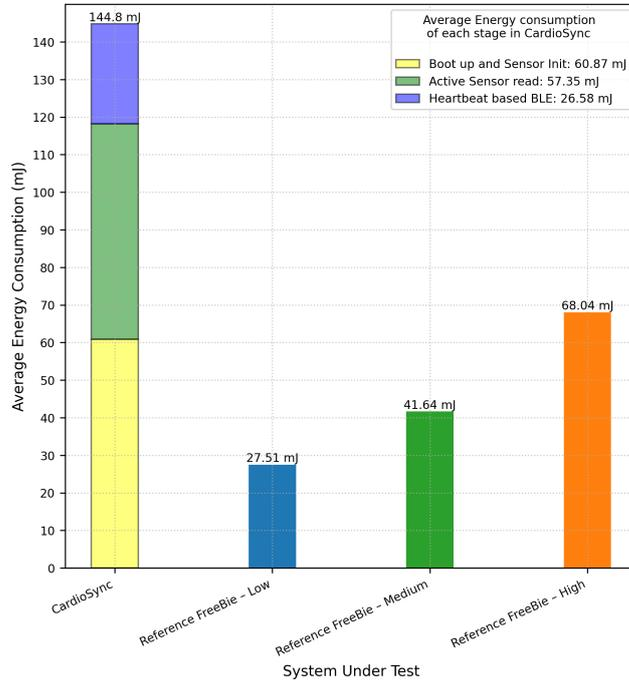
Figure 5.8: **Comparison of average energy consumed till connection setup for each system.**
