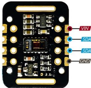
Figure 4.2: MAX30102 sensor module (front side). The pin out marked are VIN: Module power supply 1.8V to 5V; GND: Ground; SCL: I<sup>2</sup>C clock bus; SDA: I<sup>2</sup>C data bus. Figure reproduced from [29].
