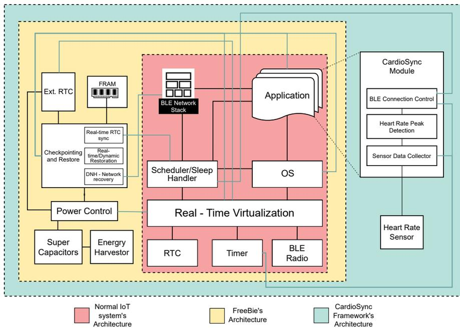
Figure 3.1: High Level Architecture of the CardioSync framework.
