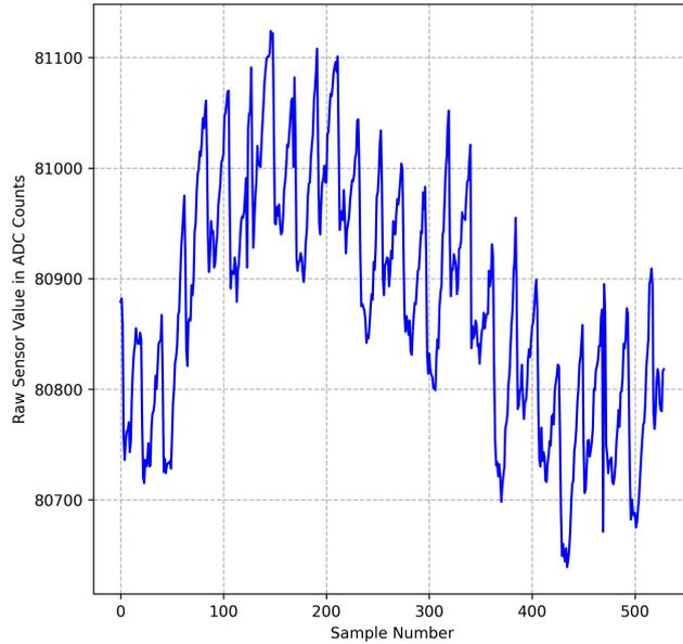
Figure 4.3: **Example measurement showing the dynamic and fluctuating nature of continuous sensor data readings from MAX30102. The Y-axis represents the sensor’s raw data in ADC count units. These units indicate the magnitude of the analog signal measured by the sensor and converted into digital form by the analog-to-digital converter (ADC).**
