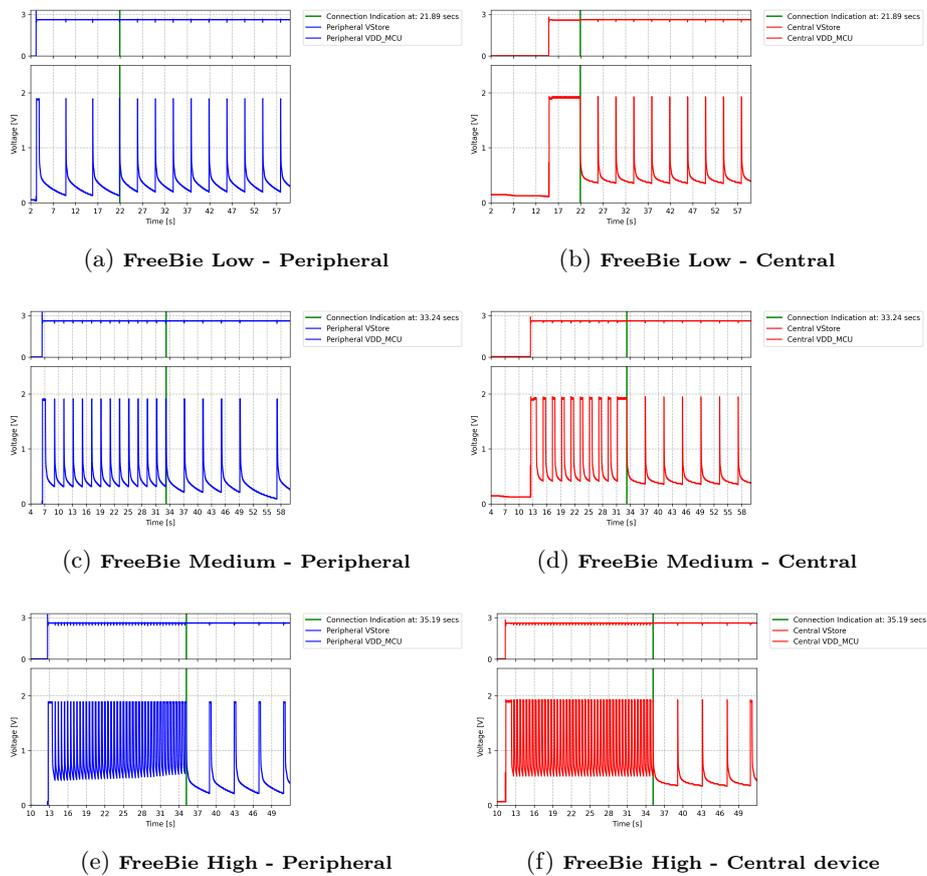
Figure 5.5: **Real-time voltage measurement of FreeBie system. Each of the two plots in both devices for each configuration shows different measurements. From top to bottom in each device, 1) Plot of  $V_{Store}$ : Supply Voltage and 2) Plot of  $V_{DD\_MCU}$ : MCU voltage. The green vertical line through all the plots indicates the successful BLE connection setup event.**
