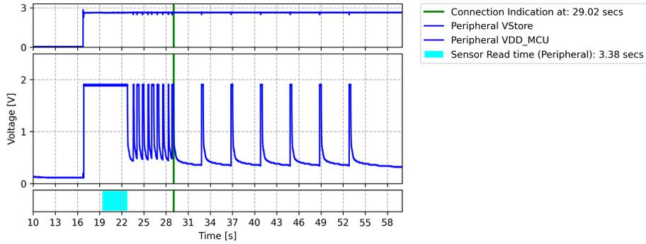
(a) Voltage measurement for peripheral device
