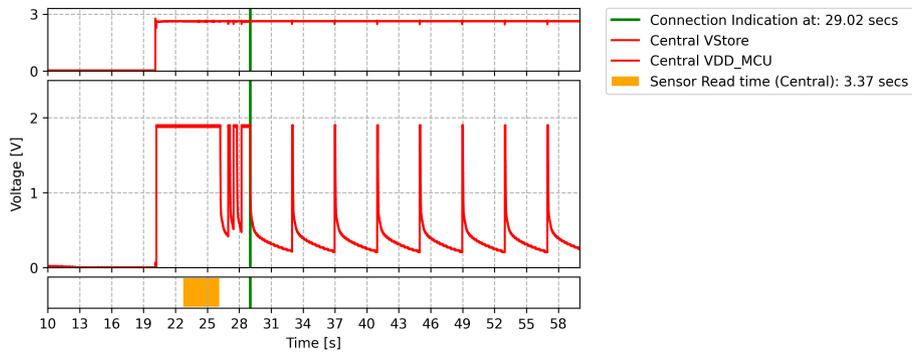
(b) Voltage measurement for central device.
