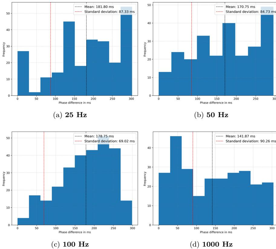
Figure 5.1: **Histograms of phase differences between heart pulses detected by two sensors at different sensor read frequencies. At 25 Hz and 50 Hz, larger phase differences occur at more frequency than 100 Hz. At 100 Hz, phase differences are evenly distributed around mean. At 1000 Hz, phases differences are more irregular.**
