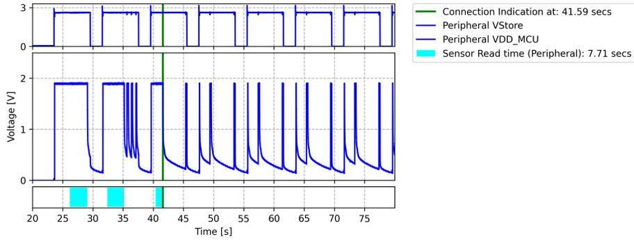
(a) Voltage measurement for peripheral device
