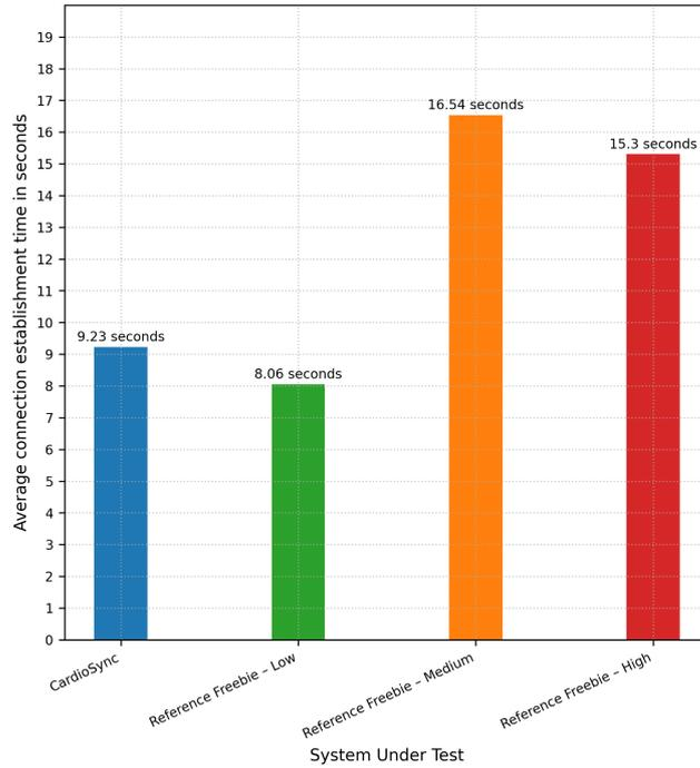
Figure 5.7: Comparison of average BLE connection establishment time for each system.
