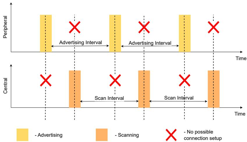
(a) Failed asynchronous periodic connection setup attempts in a FreeBie system.
