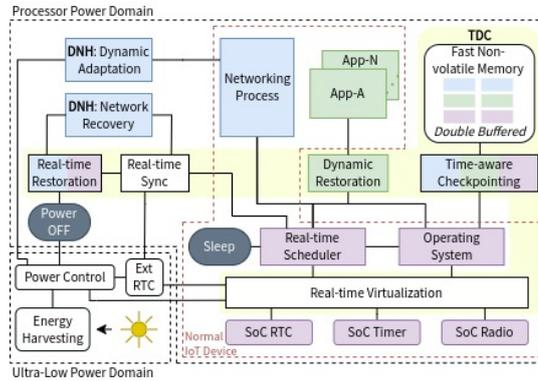
Figure 2.1: **FreeBie Architecture.** Figure reproduced from [12].
