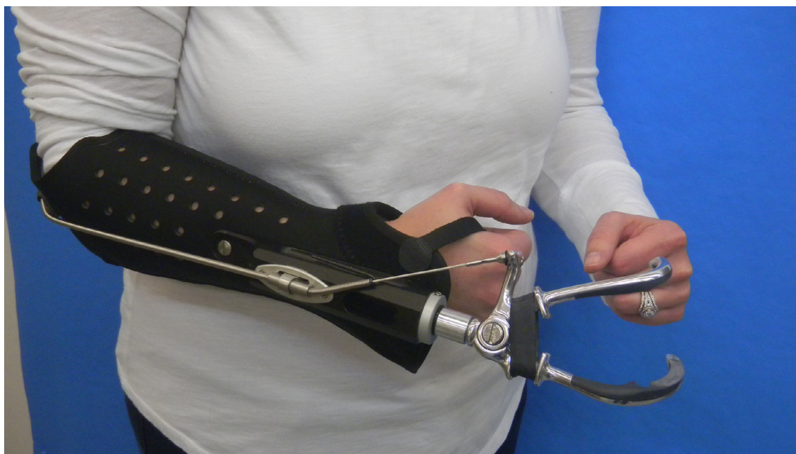
Fig. 2. Prosthesis simulators in 3 configurations (2.1: dorsal placement, Fillauer TRS [56]; 2.2: axial placement, De Boer et al. 2016 [14]; 2.3: palmar placement, Smit et al. 2015 [6]).
