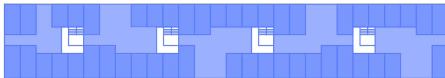
Footprint of Ekamaflat combined with Quartiershaus floorplan. More than twice as many inhabitants possible per floor
