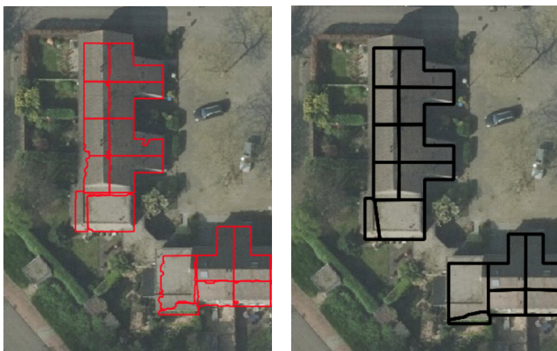
Figure 3.3: Aerial image and roof segments of Readaar, created by method for set 1 (left) and set 2 (right), gotten from [51].
