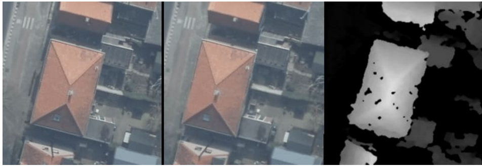
Figure 3.1: Stereo aerial images and a disparity map of a roof, gotten from Readaar [49].
