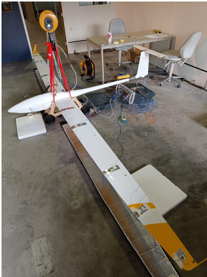
Figure 4: Ground vibration testing setup.
