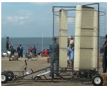
Figure 8.10: Racing Aeolus Hardliner wind car with vertical axis wind turbine (VAWT) and protection structure
