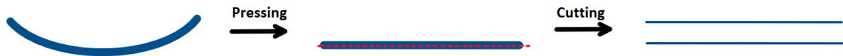
Figure 6.4: Manufacturing process to reduce the thickness. The dotted red line indicates the cutting direction.
