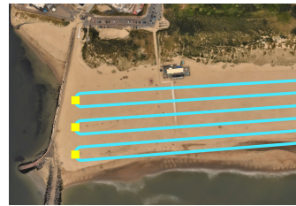
Figure 10.3: An example of predetermined obstacle avoidance using waypoints.
