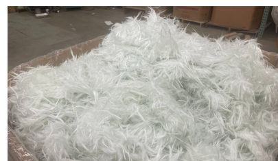
Figure 2.4: Reclaimed glass fibre from pyrolysis on blades (Carbon Rivers)
