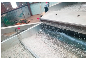
Figure 2.3: Ground up blade composites turned into pellets (Global fibreglass Solutions)
