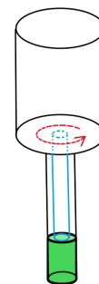
Figure 12.4: Representation of the VAWT. The blue section is the rotating shaft that carries the torque and transmits it to the generator shown in green.
