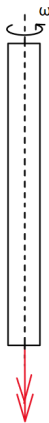
Figure 8.22: Braking torque applying to the rotating shaft provided by the disc braking system
