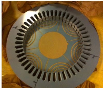
Figure 2.8 Reluctance rotor of brushless DFRM [28]
