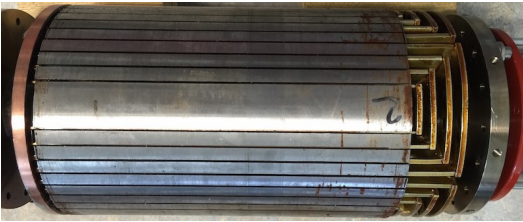
(c) Rotor 3 (big loop span, non-skewed)
