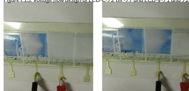
Figure I.14: ECD-C-76: Voltage flow.
