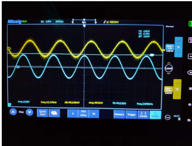
Figure 8.3: Resonance shown on oscilloscope with input (yellow) and output (blue) signal.
