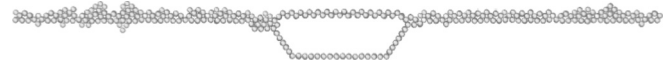
FIG. 16. Contact with nanoscale asperities for case AB. Atoms that do not belong to the interface, i.e., that have fcc structure type, are excluded.
