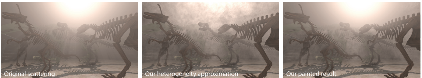
Fig. 18. Heterogeneity modification. From left to right: the original scattering produces regular light shafts; heterogeneity is approximated using a 3D Perlin noise texture, which creates more irregular scattering effects and gives the medium a distinguishable volumetric structure; using our 3D painting tool, we can remove unwanted details that are due to heterogeneity while retaining the irregularity of the light shafts.
